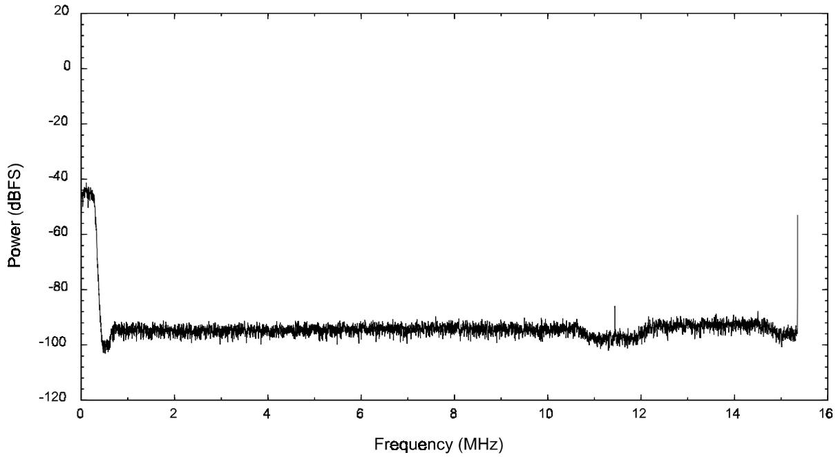
Figure 6. Self generated spurious response averaged power spectrum.
