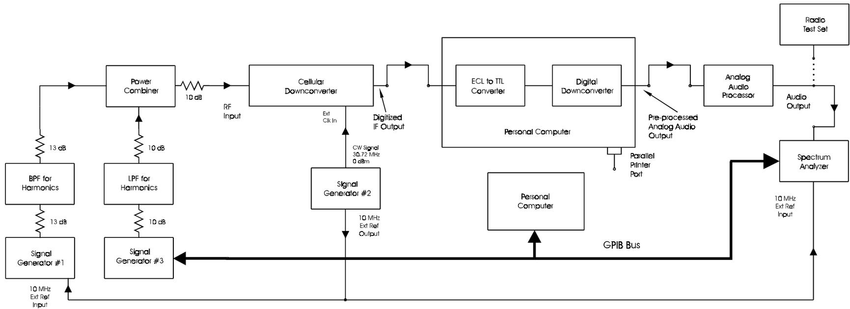
Figure 22. Test setup for the first stage of the spurious response interference test (for 0.68 - 550 MHz interfering signals).
