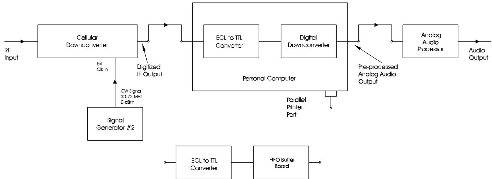
Figure 1. Architecture of the entire configuration of the cellular B-band receiver.
