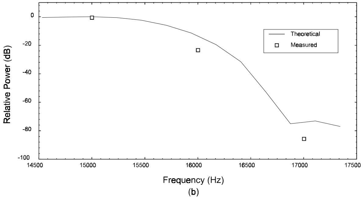
Figure 17. Measured and theoretical (a) passband and stopband and (b) transition band frequency response of the channel filter.
