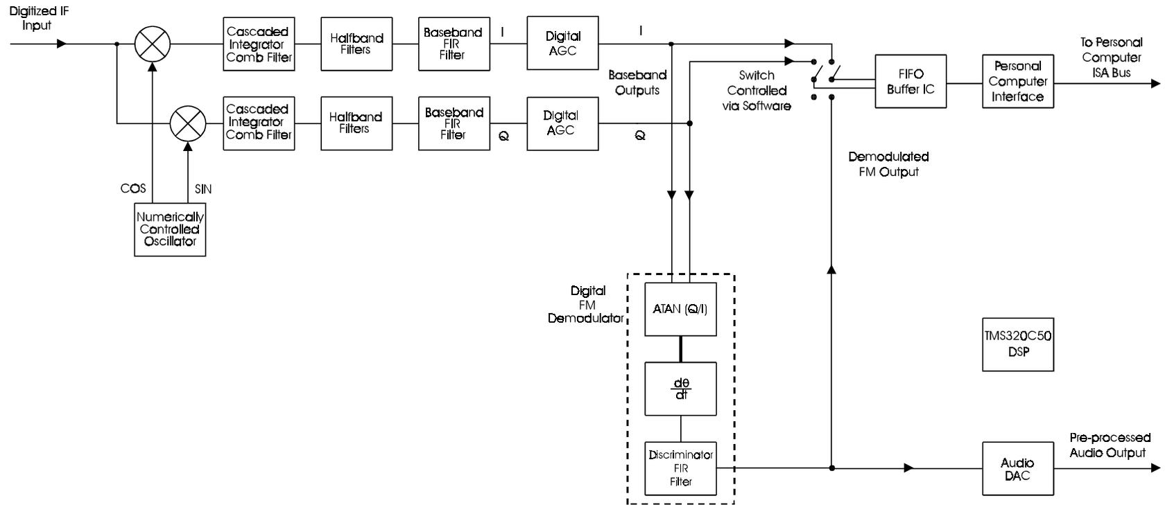
Figure 2. Processing performed by the digital downconverter.
