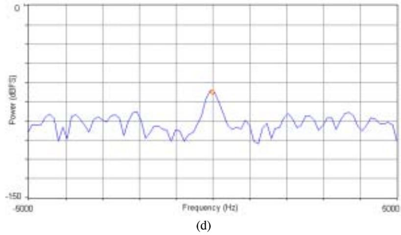
Figure 19. Output baseband spectrum with digital AGC disabled for 840-MHz RF input signal levels of (a) -15, (b) -40, (c) -60, and (d) -110 dBm.
