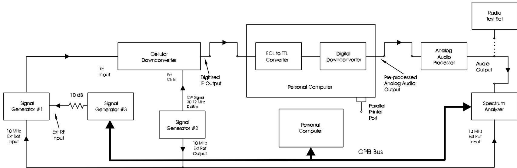
Figure 23. Test setup for the first stage of the spurious response interference test (for 1000 - 2600 MHz interfering signals).
