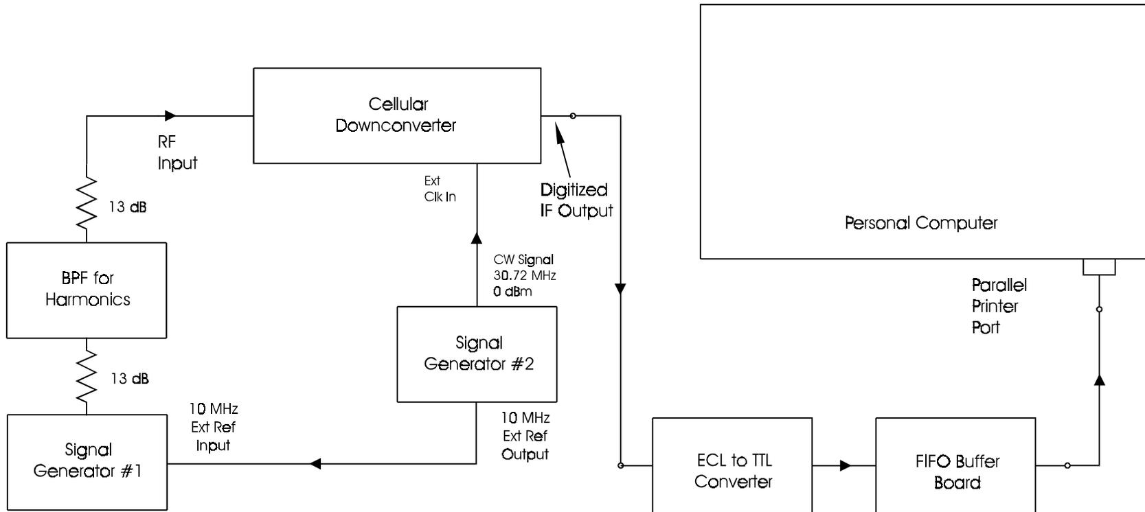
Figure 5. Test setup and receiver configuration to observe the digitized IF output.
