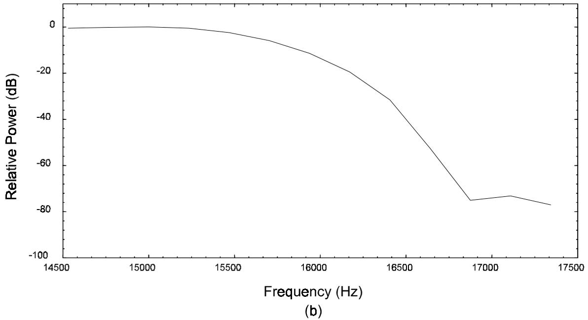
Figure 4. Magnitude response of the baseband FIR filter showing the (a) passband and stopband and (b) transition band.
