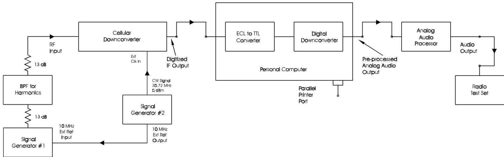
Figure 21. Test setup for the audio output channel desensitization test.
