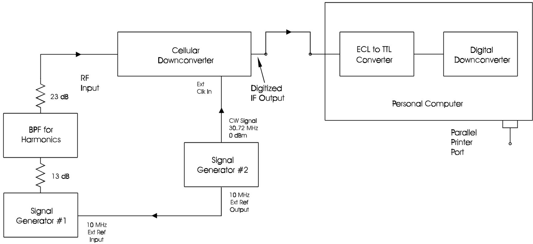
Figure 15. Test setup for observing the receiver baseband and demodulator outputs.
