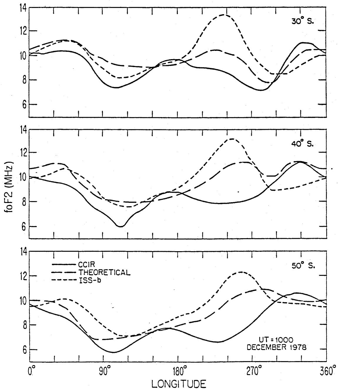
Figure 17. Longitudinal distribution of foF2 at 30°, 40°, and 50° south latitude for December 1978 at 1000 hrs UT.
