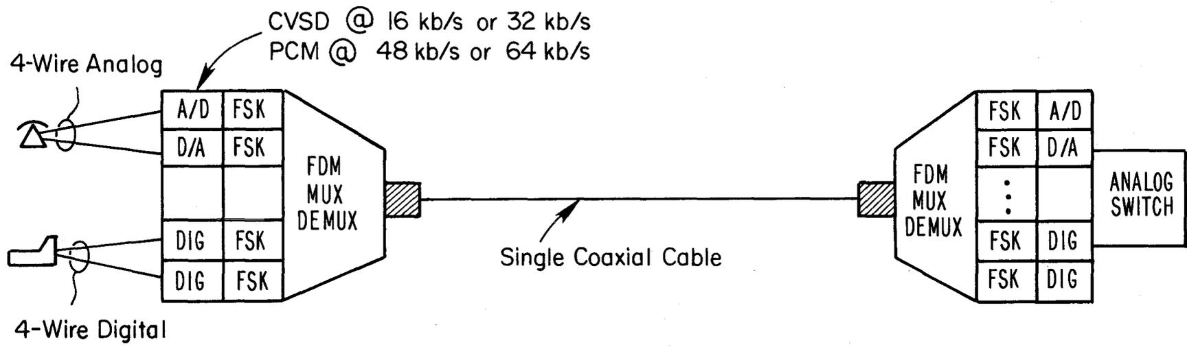
Figure 73. CP/SC Alternative IV canonical bus distribution system.
