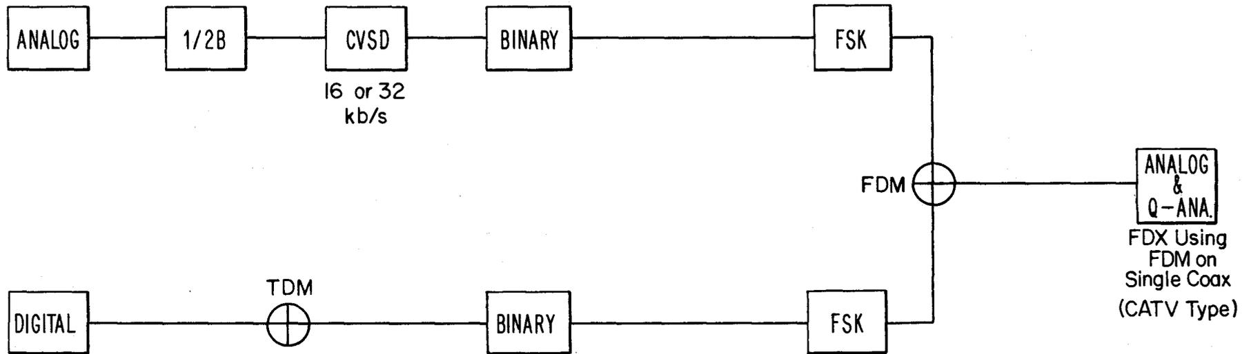
Figure 72. Alternative IV for CP/SC link structure.
