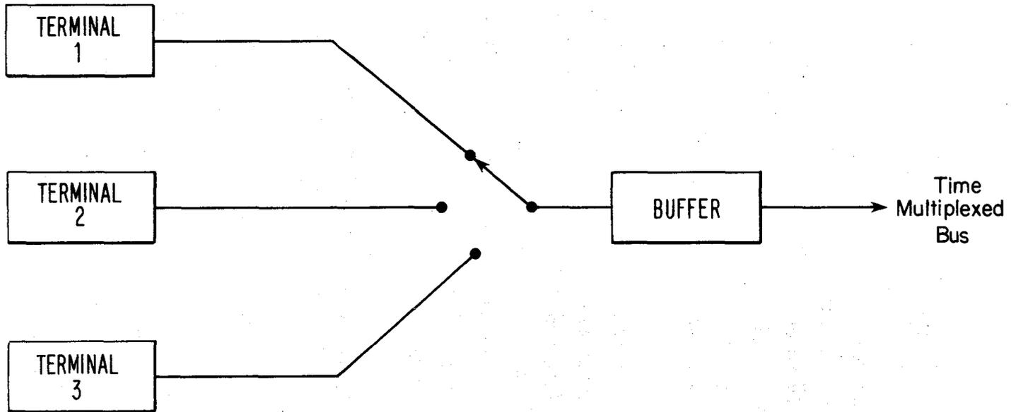
Figure 17. Synchronous time division multiplexer.
