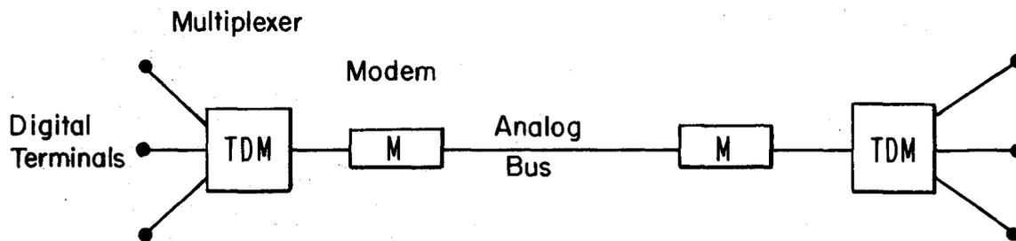
Figure 55. Multiplexing digital terminals on an analog bus.
