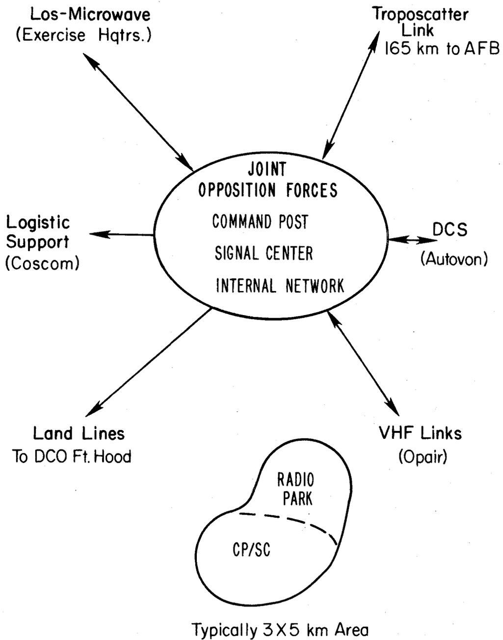
Figure 6. External traffic links to command post used for operation Braveshield exercise.
