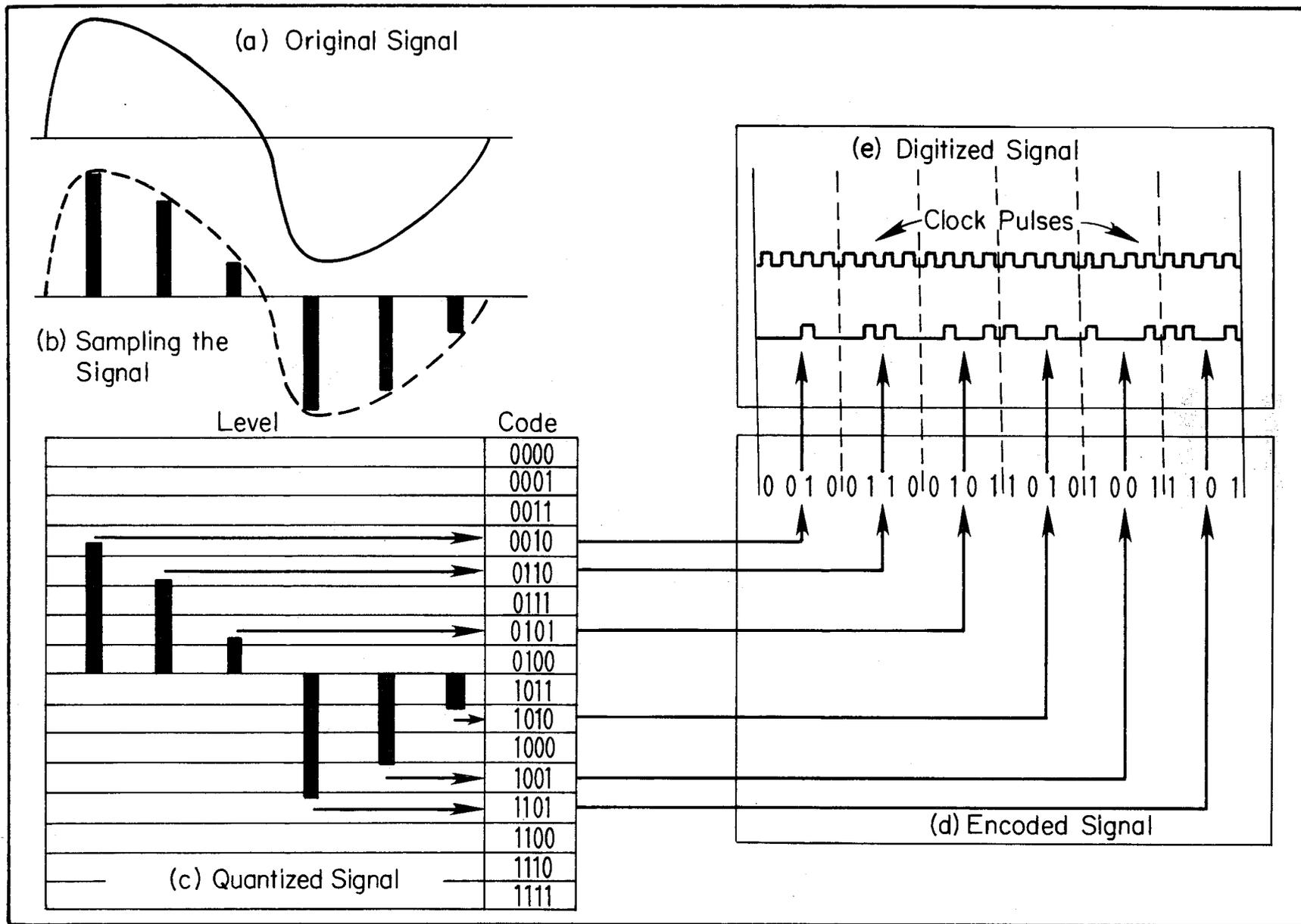
Figure 50. Steps in pulse coding an analog signal.
