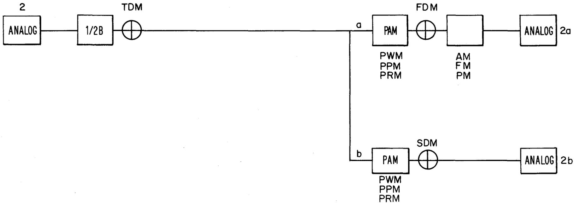
Figure 61. Transparent bus structures for time discrete analog signals.
