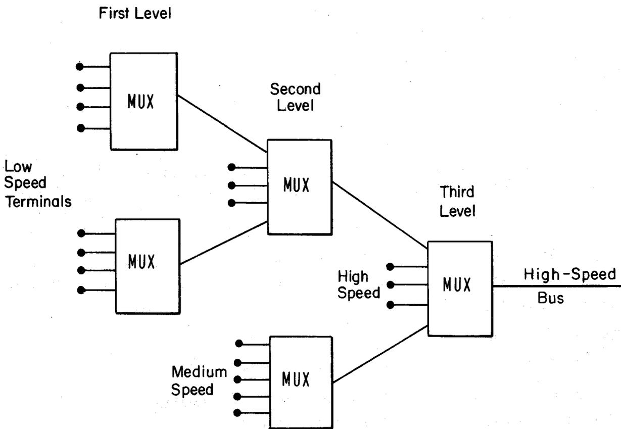
Figure 57. Multiplexing terminal with different source rates.
