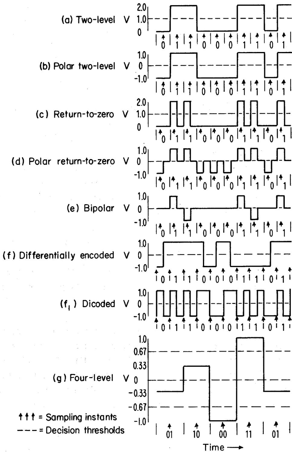
Figure 51. Common digital signal formats for transmission.
