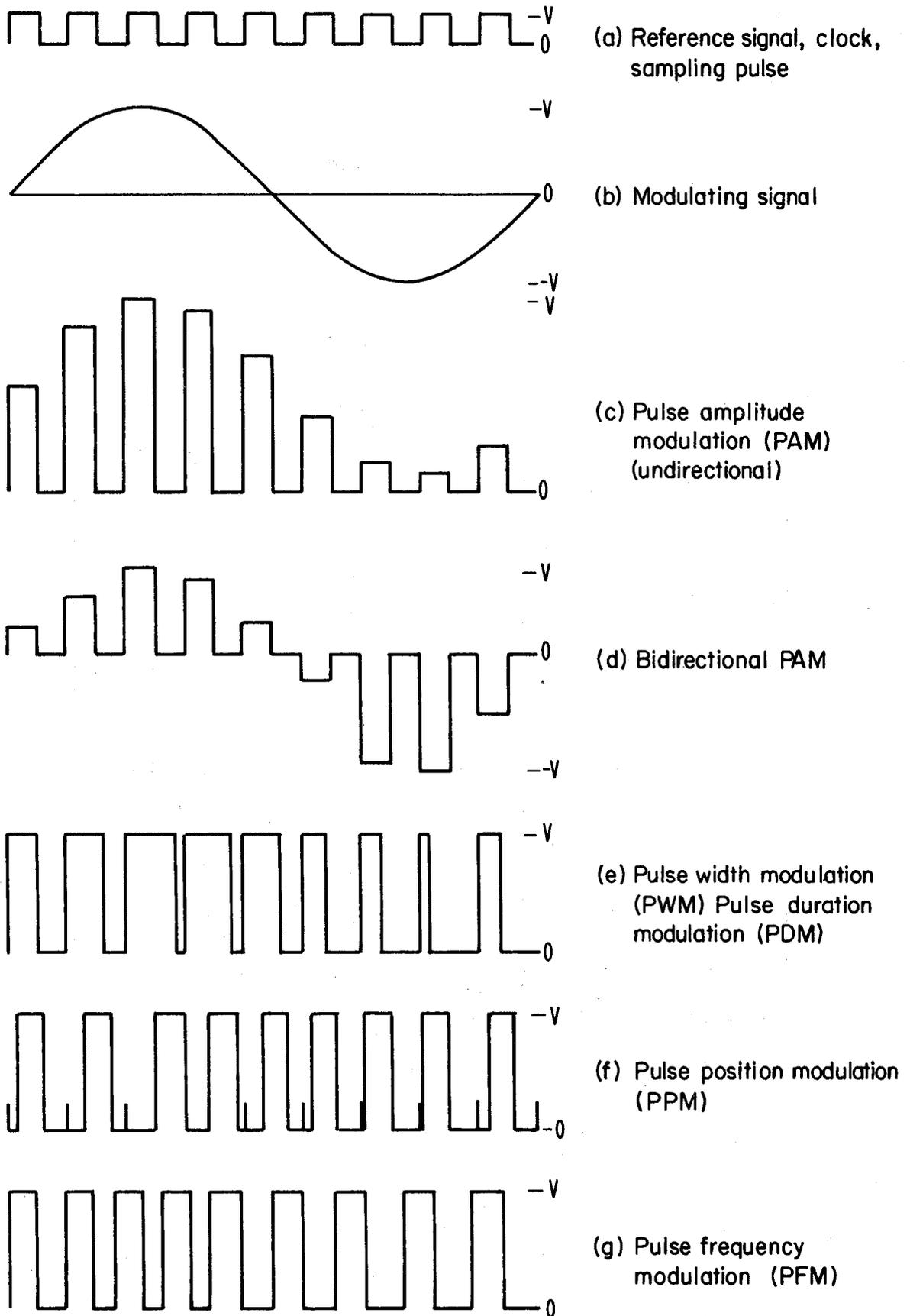
Figure 53. Noncoded pulse waveform representations.
