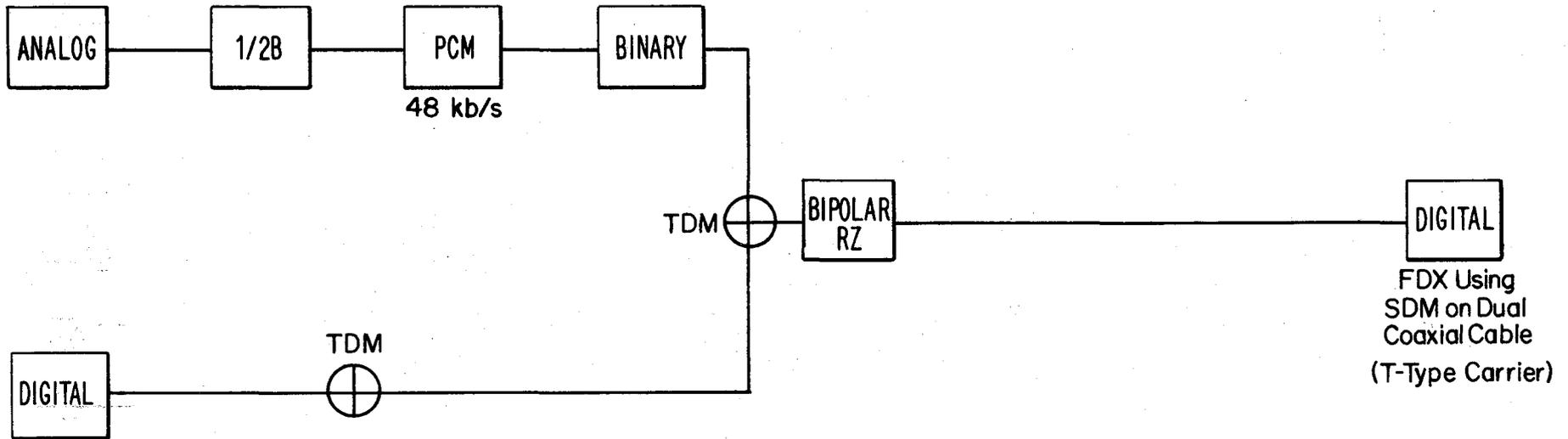
Figure 70. Alternative III for CP/SC link structure.
