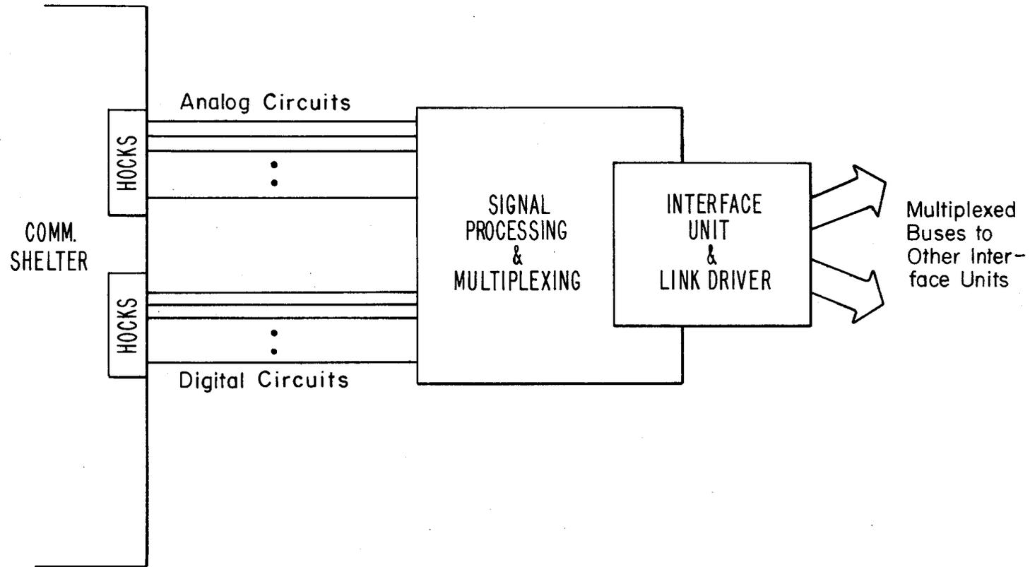
Figure 48. Transparent link structure for demonstrating technical feasibility of bus-type network.
