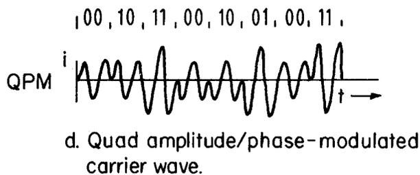
Figure 52. Common modulated carrier signals.
