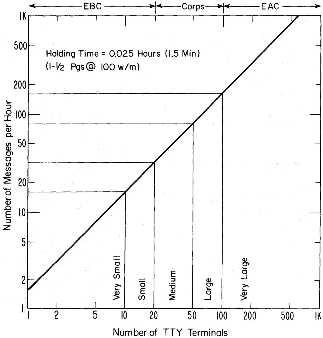
Figure 13. CP/SC size relationships for teletype terminals and message/hour.
