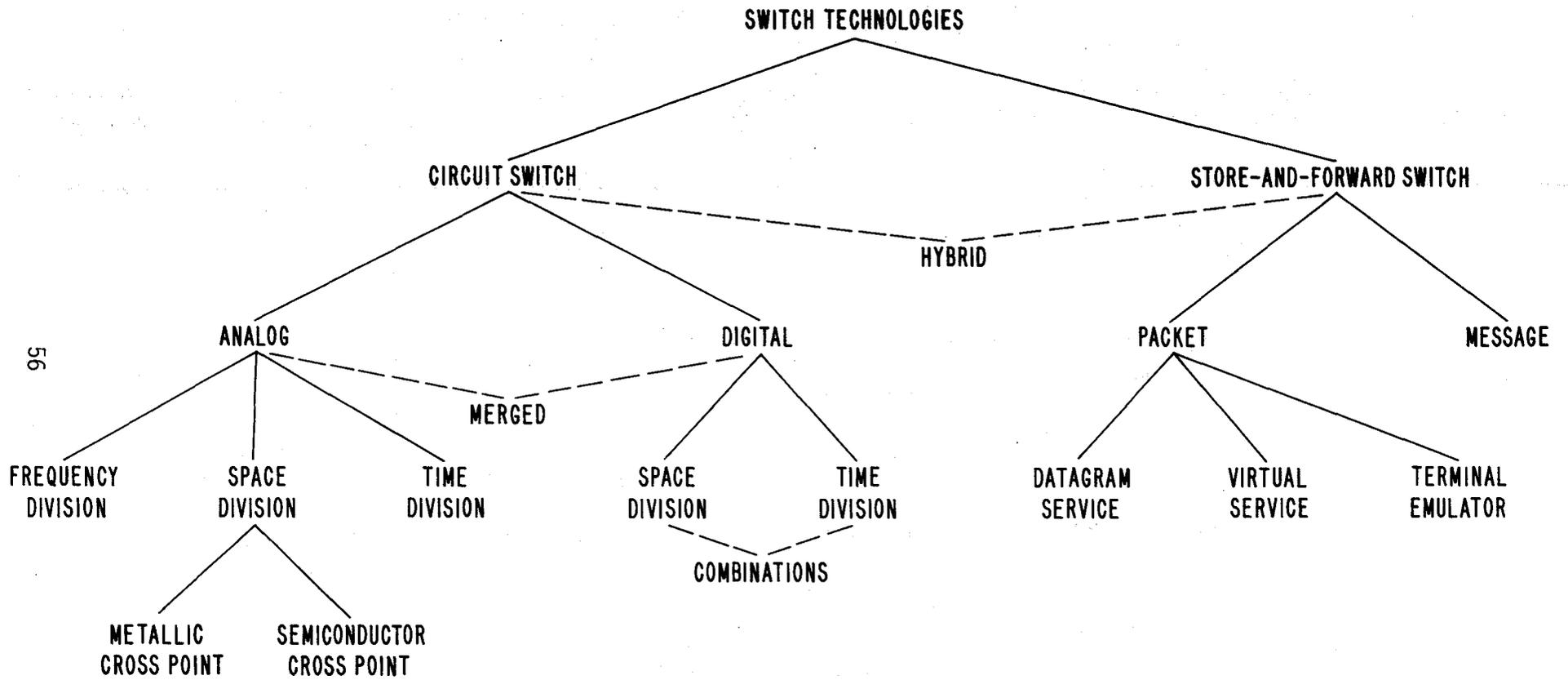
Figure 18. Switch technology classifications.
