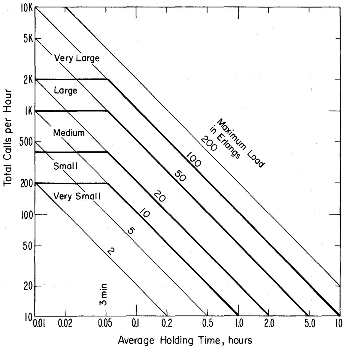
Figure 12. CP/SC size relationships in terms of maximum telephone traffic load.
