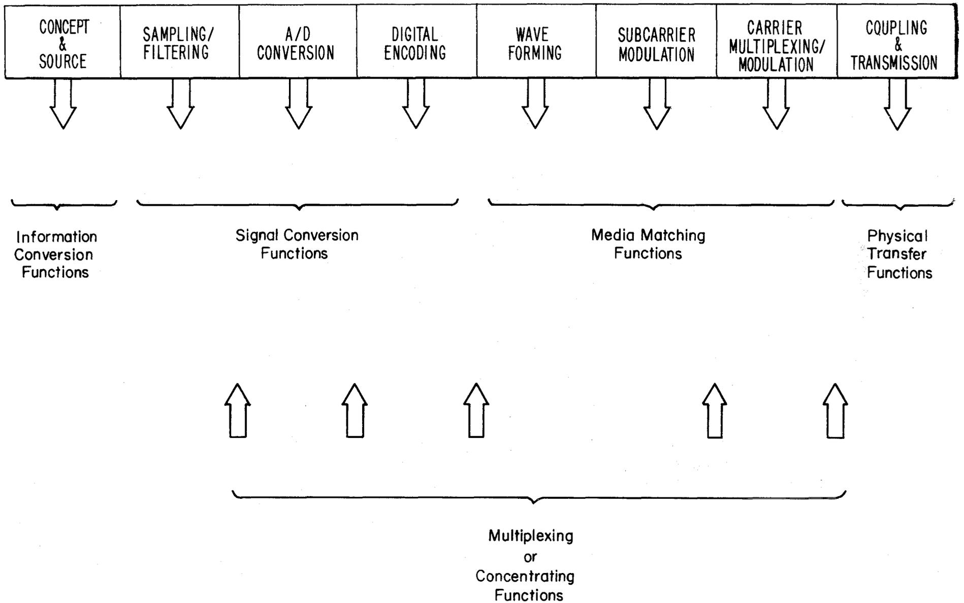
Figure 49. Basic communications functions.
