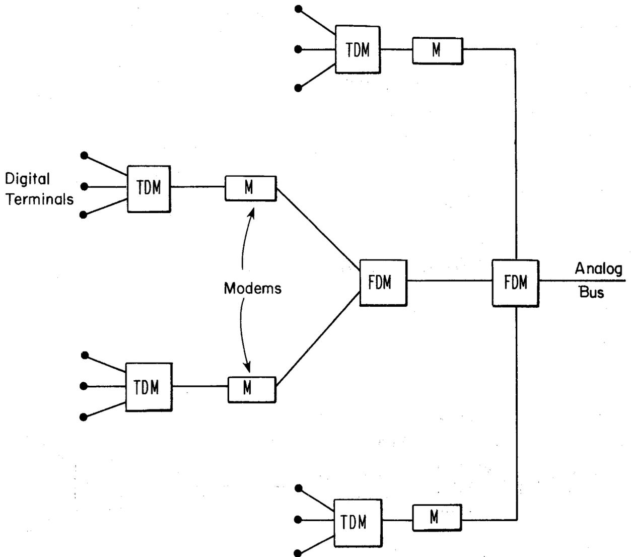
Figure 56. Multiplexing digital terminals on an analog bus with separated access.
