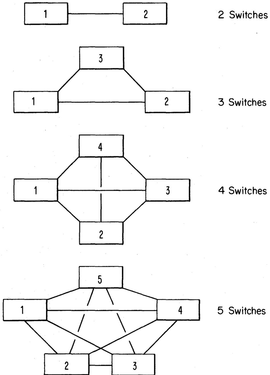
Figure 33. Fully interconnected, distributed switch hierarchy level.
