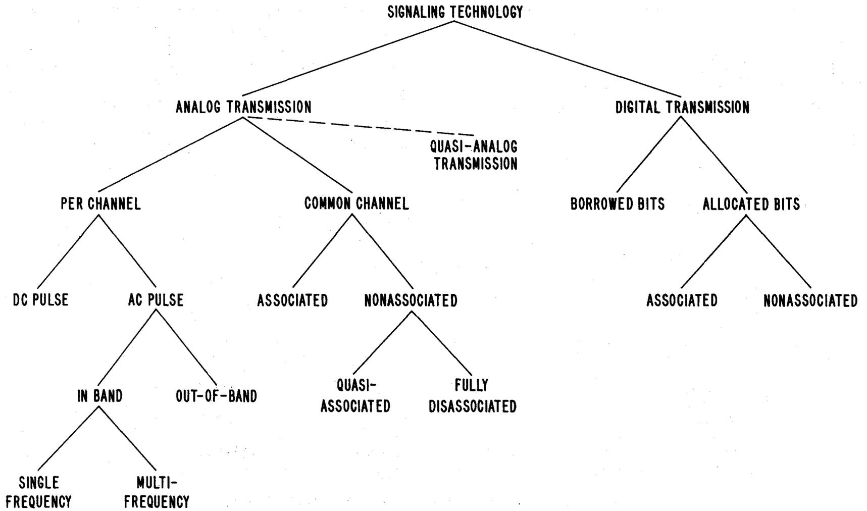
Figure 20. Signaling technologies for remote switch control.
