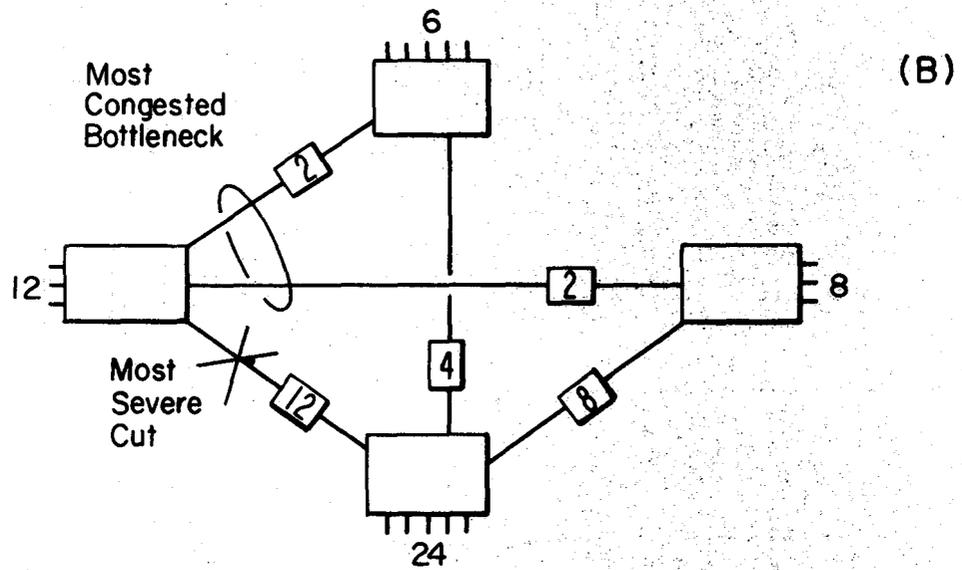
Figure 42. The most severe cuts and bottlenecks in simple networks.
