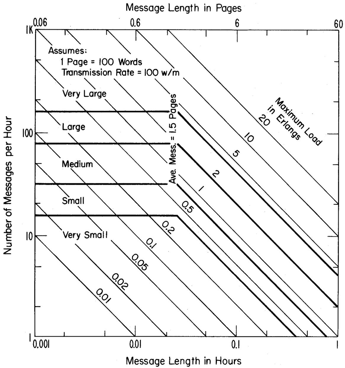
Figure 14. CP/SC sizing based on maximum teletype traffic.
