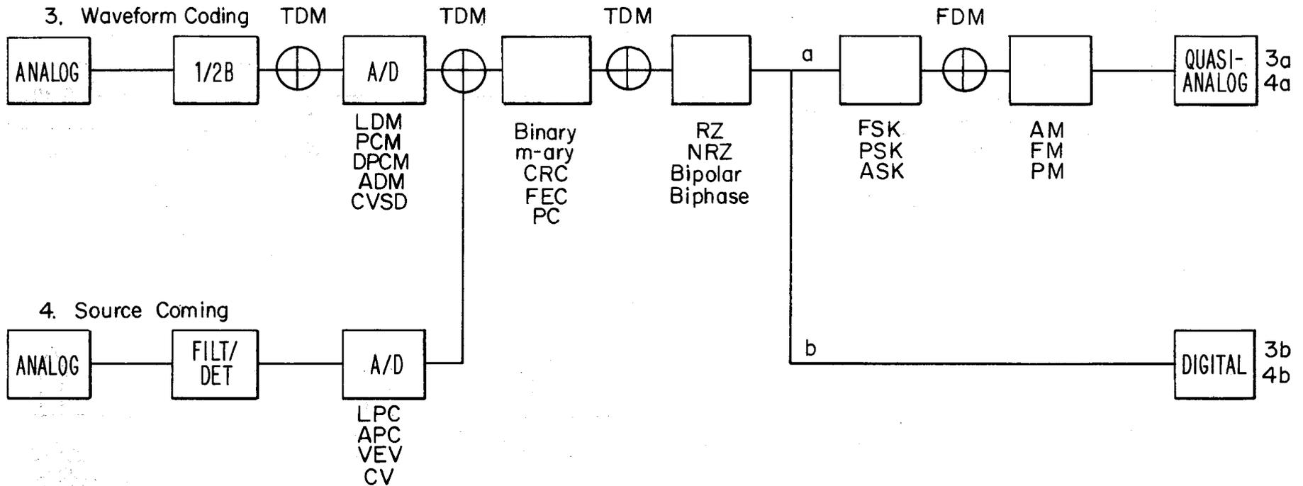
Figure 62. Transparent bus structures for digitized analog signals.
