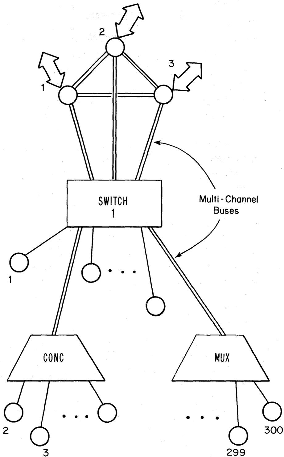
Figure 32. A four-level hierarchy with centralized switching.
