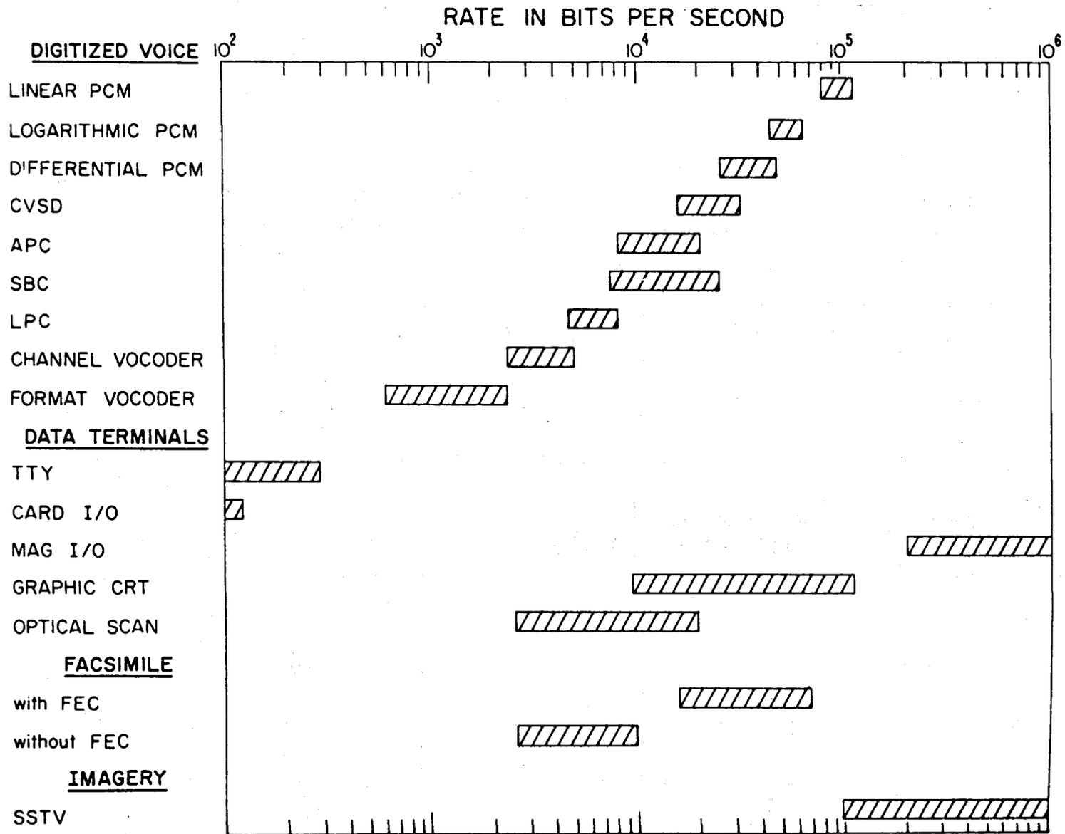
Figure 10. Traffic rates generated by various types of terminals.
