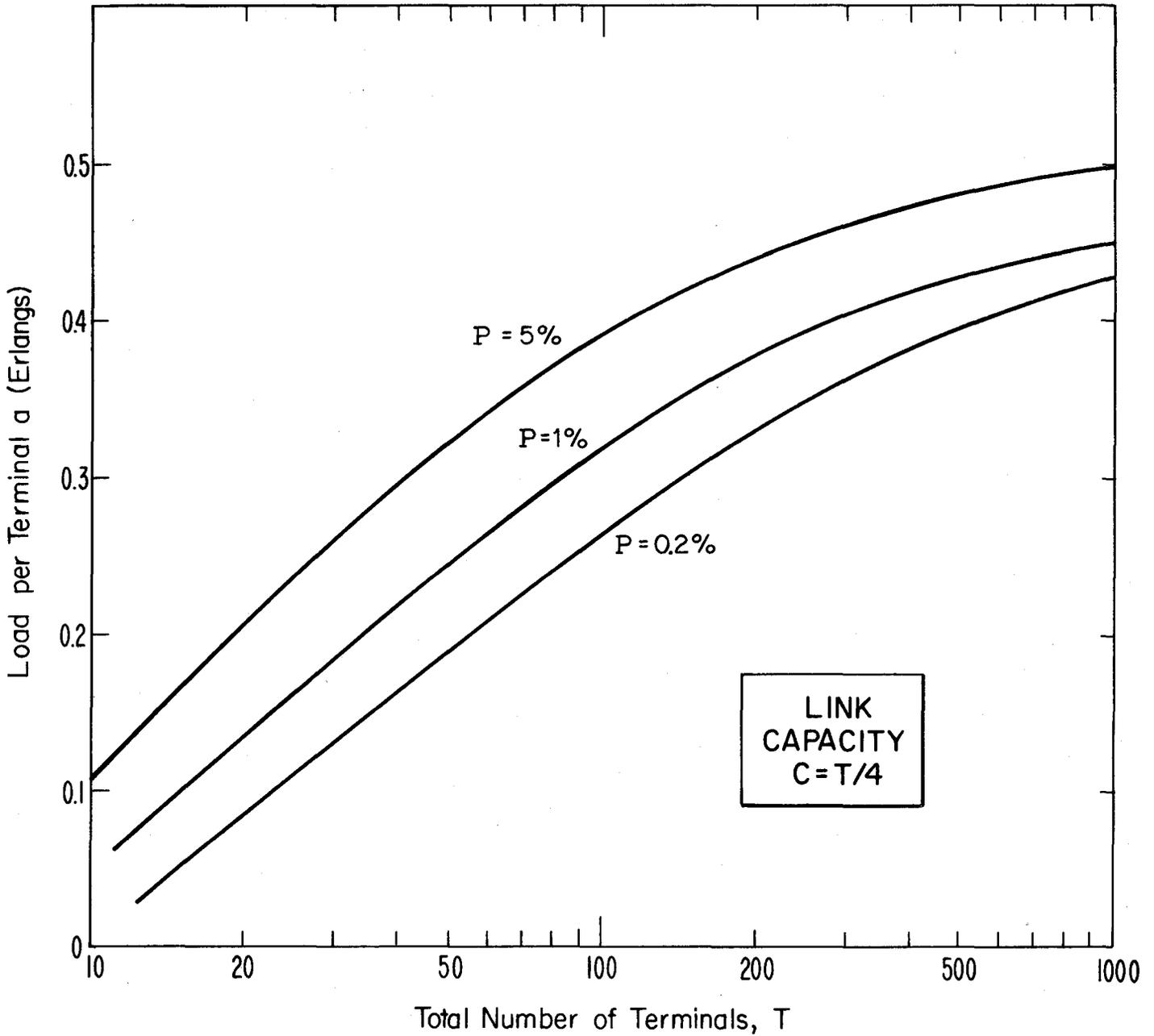
Figure 41. Worst case probability of blocking for the uniform loop network with a single link outage.
