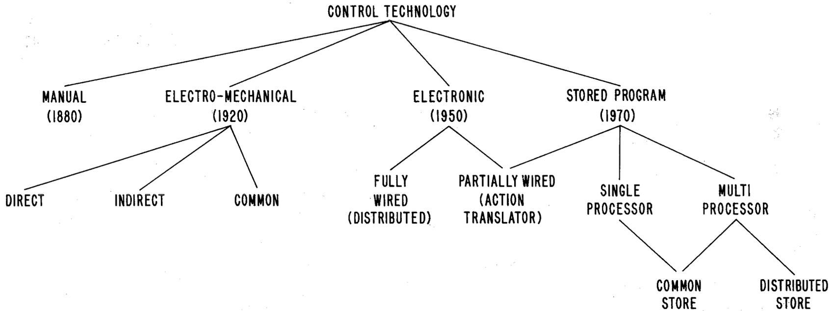
Figure 19. Control technologies used in circuit switching systems.
