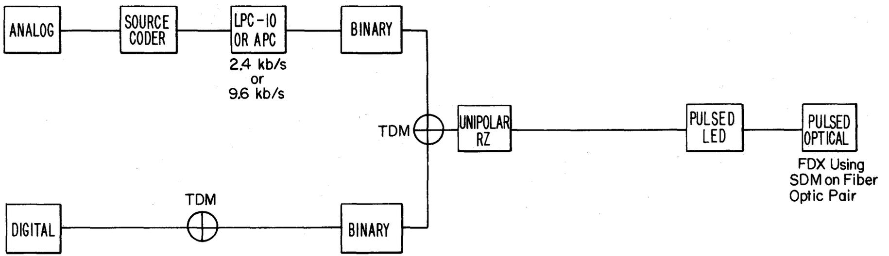
Figure 74. Alternative V for CP/SC link structure.
