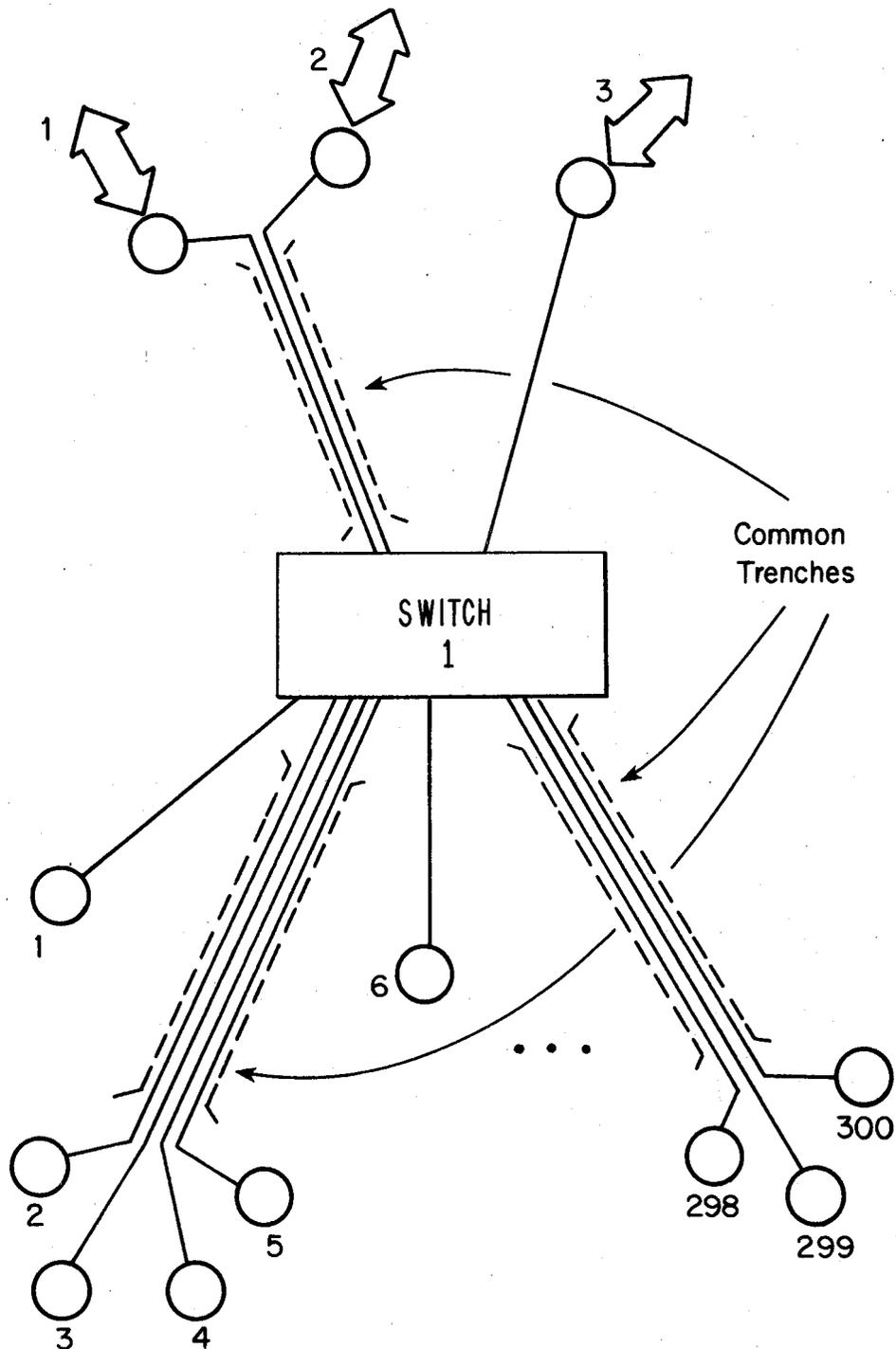
Figure 31. Space-division-multiplexing (SDM) or common trenches for the star network.
