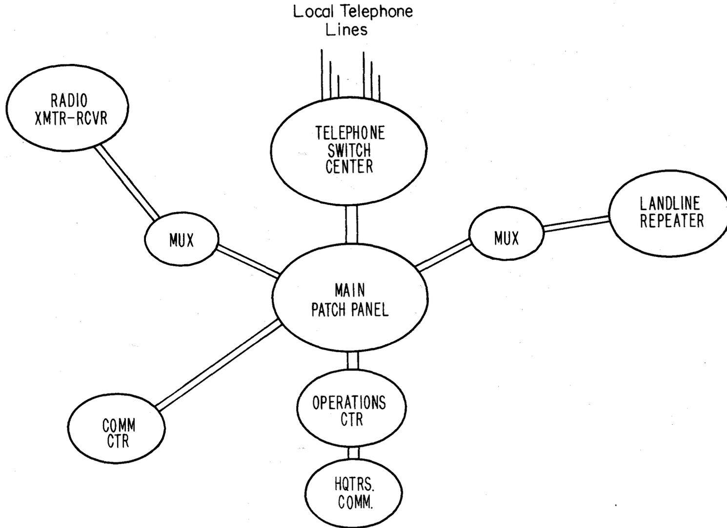
Figure 5. Interconnection of functional units for a typical area signal center.
