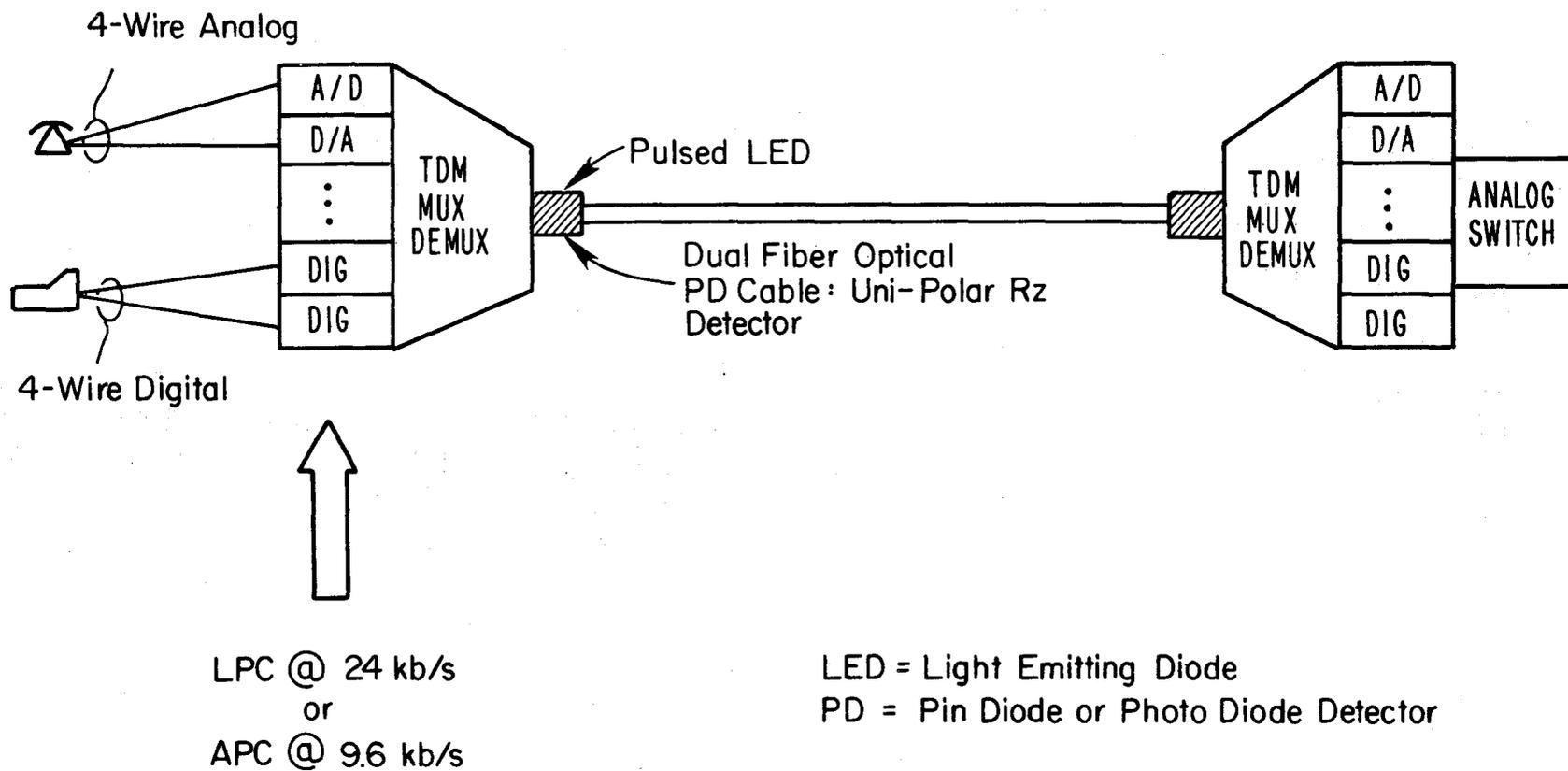
Figure 75. CP/SC Alternative V bus distribution system.
