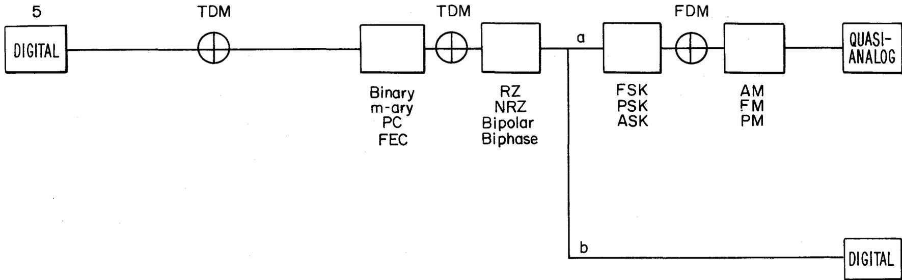
Figure 63. Transparent bus structures for digital signals.
