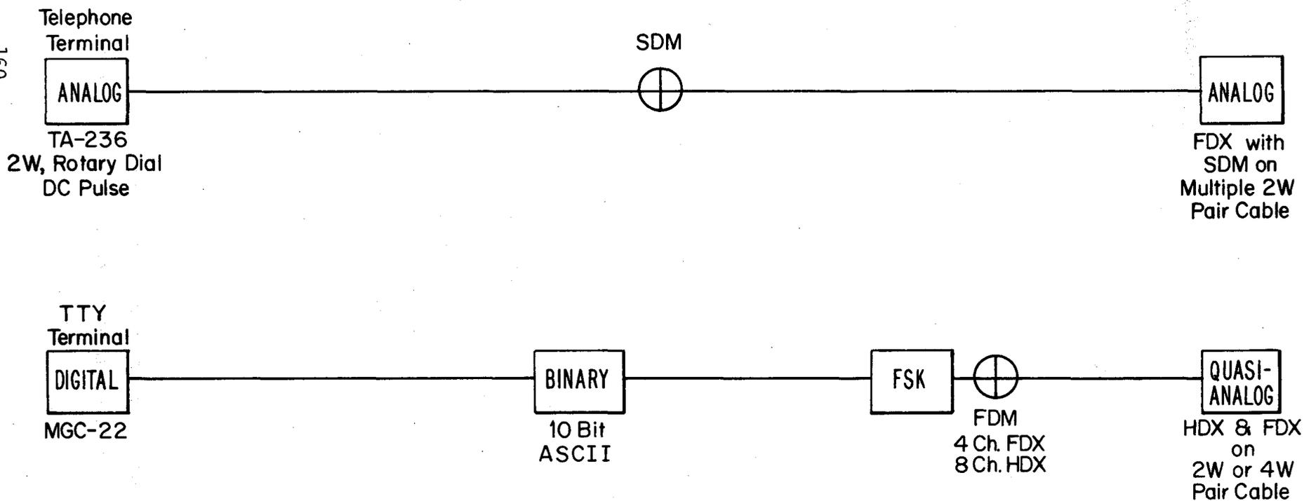
Figure 64. Existing CP/SC link structure.
