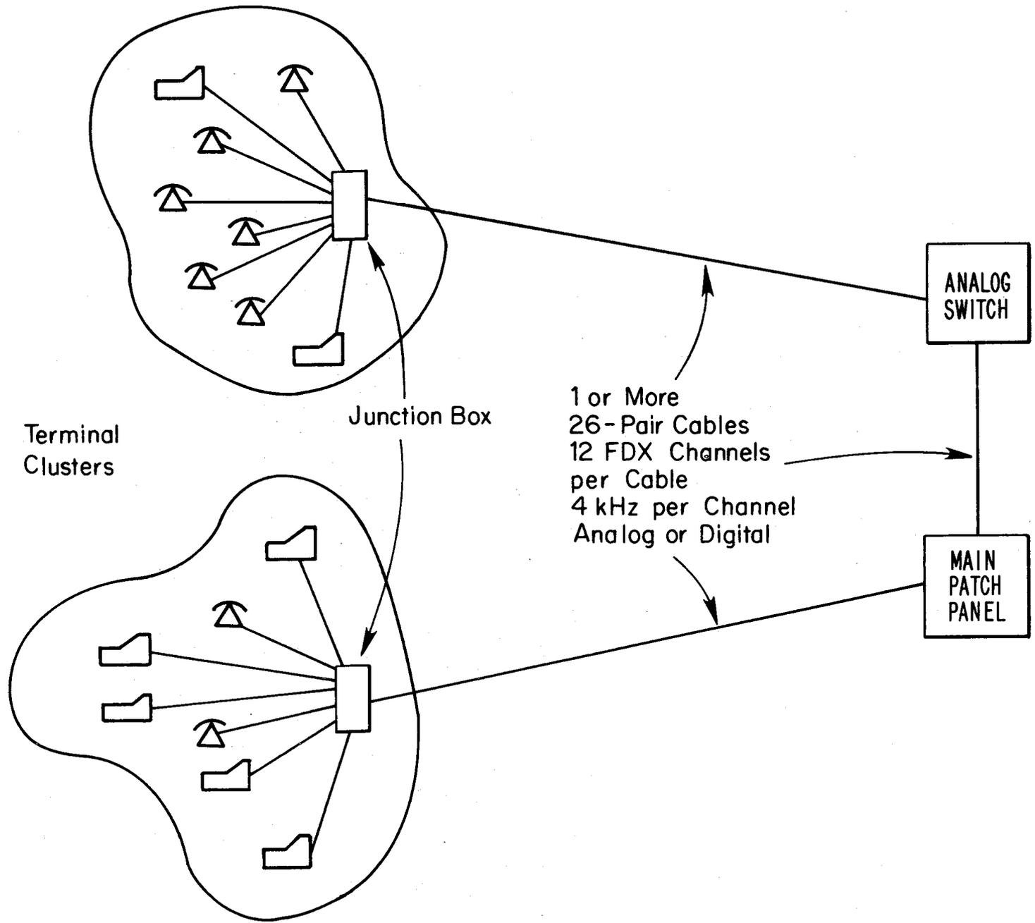
Figure 65. Existing CP/SC cable run structure.
