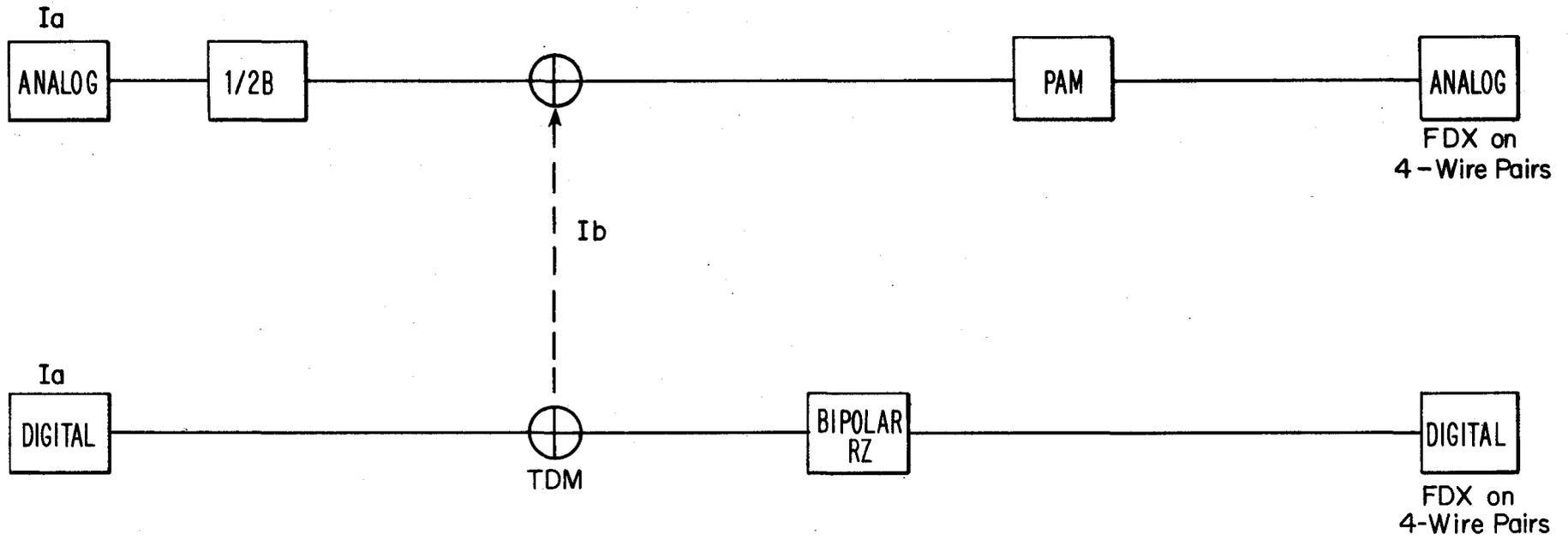
Figure 66. Alternative I for CP/SC link structure.
