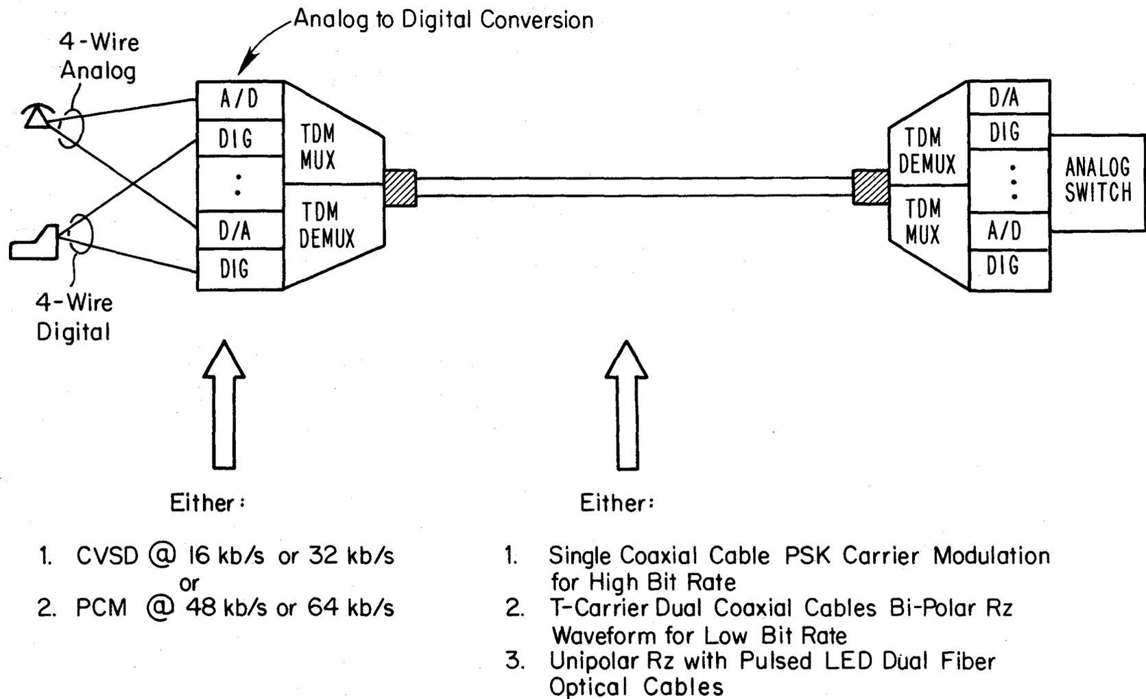
Figure 71. CP/SC Alternative III canonical bus distribution system.
