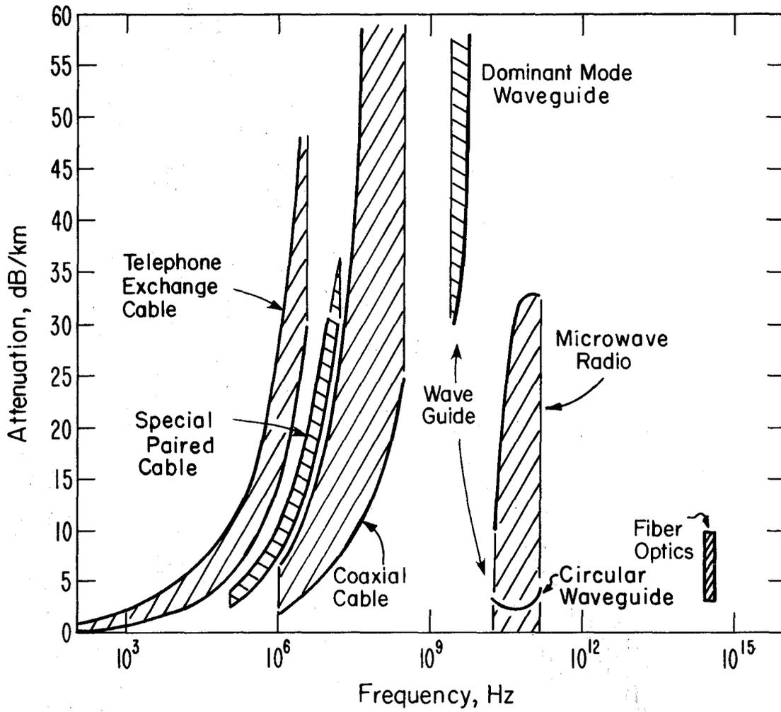
Figure 58. Losses of current telecommunication media.
