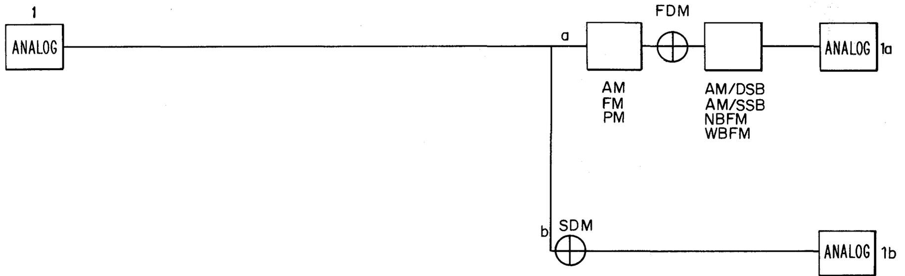
Figure 60. Transparent bus structures for time continuous analog signals.
