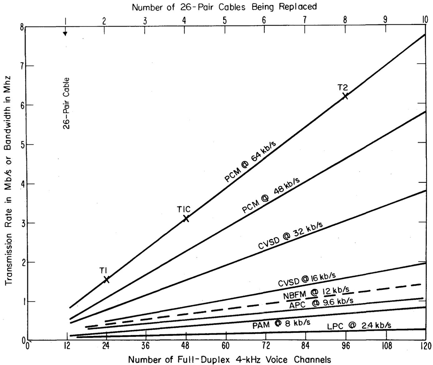
Figure 76. Estimates of bus channel capacity for various bus distribution systems.
