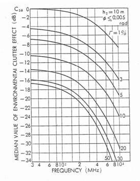
Figure 3. Median value of clutter effect as a function of frequency. From Kinase (1969).
