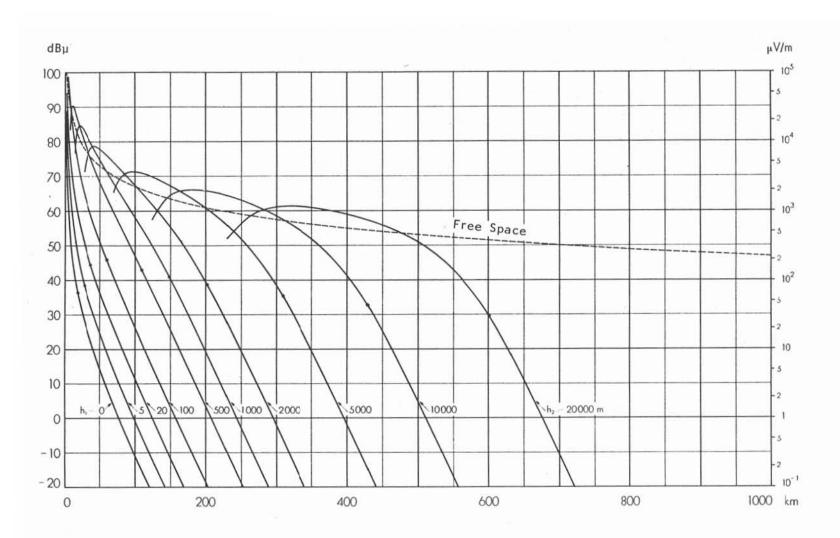
Figure A-1. Field strength (for 1 kW ERP) as a function of distance over a smooth homogeneous earth. Frequency 100 MHz,  $\varepsilon = 10$ ,  $\sigma = 10$  mS/m,  $h_1 = 20$  m,  $h_2 = 0$  to 20,000 m.
