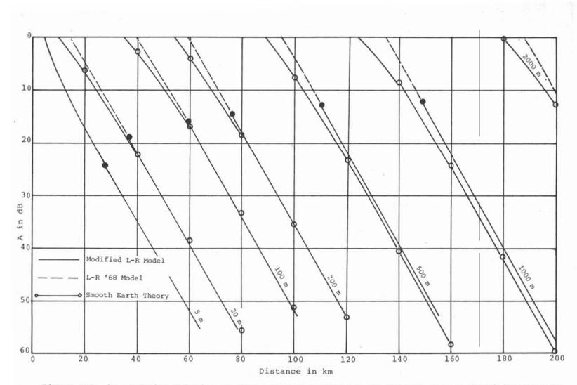
Figure A-4. Attenuation relative to free space as a function of distance over a smooth homogeneous earth. Frequency 1000 MHz,  $\varepsilon = 15$ ,  $\sigma = 5$  mS/m,  $h_1 = 20$  m,  $h_2 = 5$  to 2000 m.
