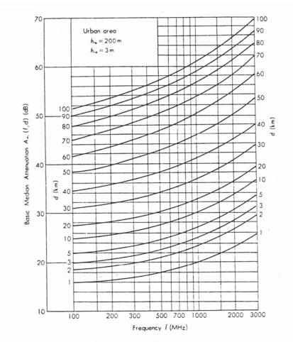
Figure 1. Prediction curve for basic median attenuation relative to free space in urban area over quasismooth terrain, referred to h = 200 m, h = 3 m. From Okumura et al. (1968).
