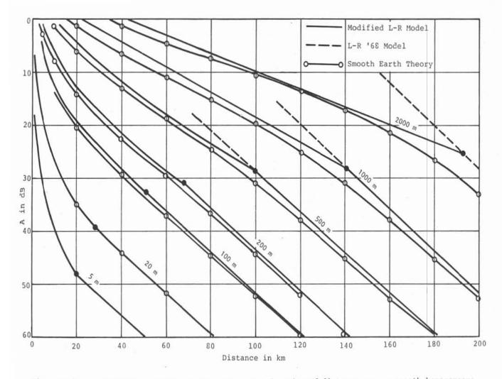
Figure A-2. Attenuation relative to free space as a function of distance over a smooth homogeneous earth. Frequency 100 MHz,  $\epsilon$  = 15,  $\sigma$  = 5 mS/m,  $h_1$  = 5 m,  $h_2$  = 5 to 2000 m
