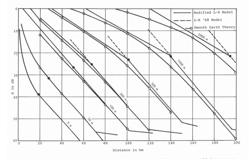
Figure A-3. Attenuation relative to free space as a function of distance over a smooth homogeneous earth. Frequency 300 MHz,  $\varepsilon = 15$ ,  $\sigma = 5$  mS/m,  $h_1 = 5$  m,  $h_2 = 5$  to 2000 m.
