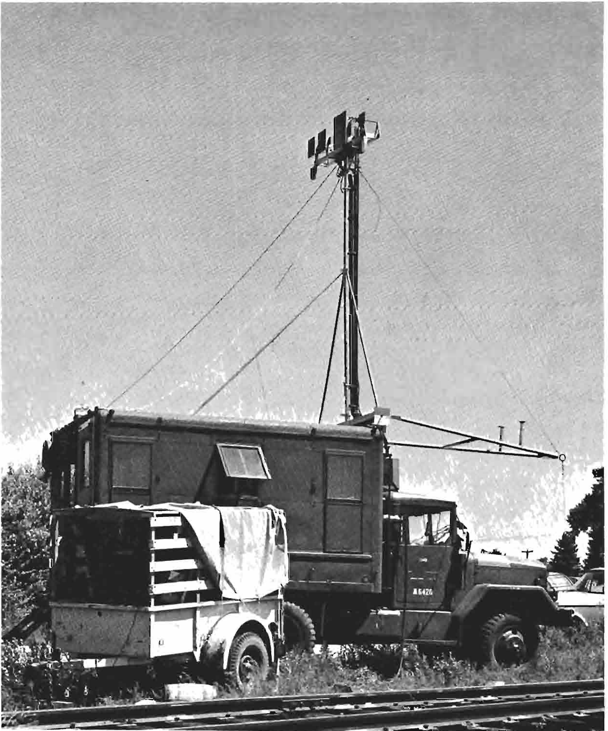
FIGURE 12 TRANSMITTING UNIT UPPER FREQUENCY GROUP
