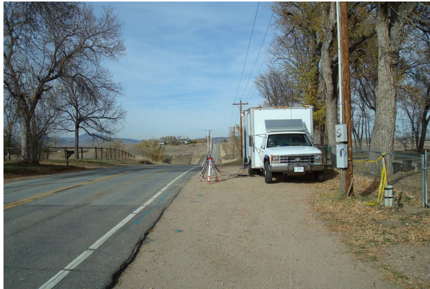
Figure 45: Short propagation path and ITS transmitter van on 63rd Street.
