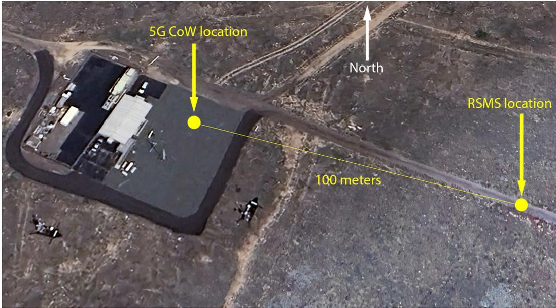
Figure 16. 5G base station CoW and RSMS geometry at Table Mountain.
