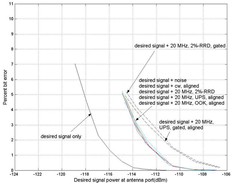
Figure 4.9. Percent bit-error versus variable LMR power for Receiver B in P25 mode – 20-MHz PRF UWB interference.
