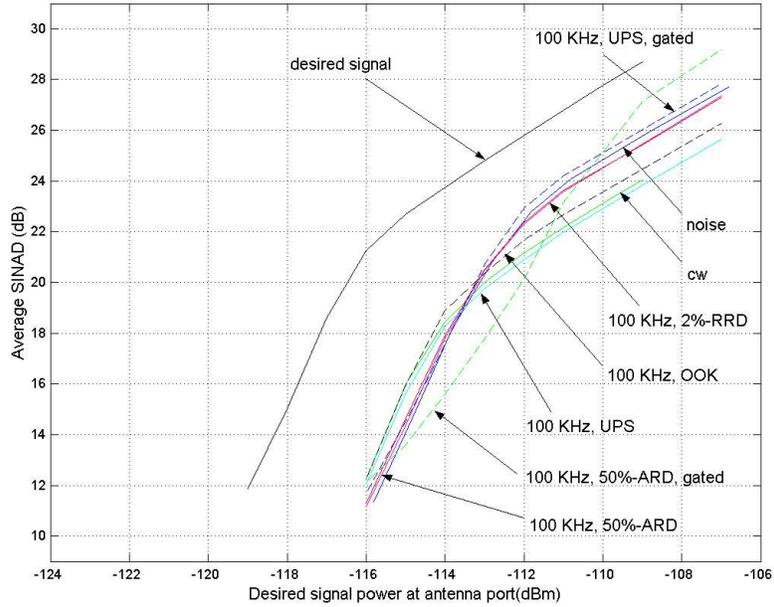
Figure 4.12. Average SINAD versus variable LMR power for Receiver B in analog mode – 100-kHz PRF UWB interference.
