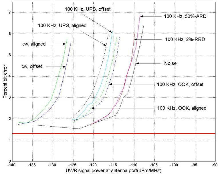
Figure 4.2. Percent bit-error versus variable interference power density for Receiver A in P25 mode – 100-kHz PRF UWB interference.
