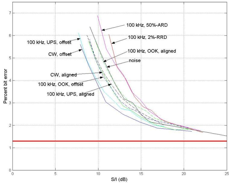
Figure 4.14. Percent bit-error versus S/I for Receiver A in P25 mode – 100-kHz PRF UWB interference.
