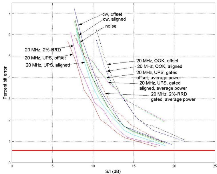
Figure 4.17. Percent bit-error versus S/I for Receiver B in P25 mode – 20-MHz PRF UWB interference.
