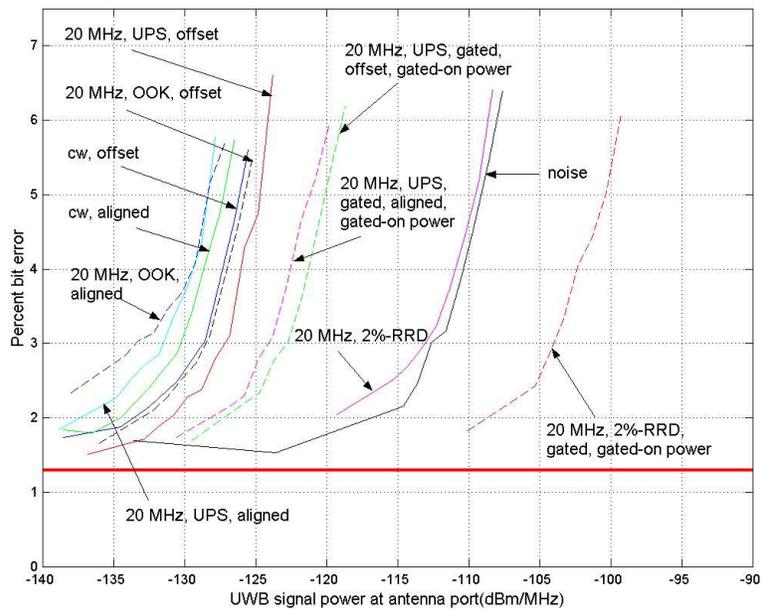
Figure 4.3. Percent bit-error versus variable interference power density for Receiver A in P25 mode – 20-MHz PRF UWB interference.
