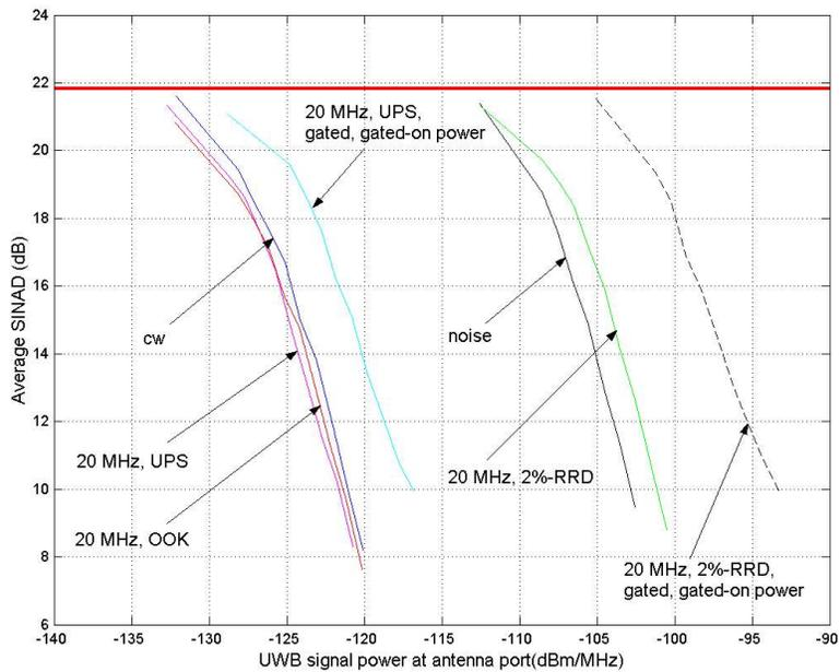
Figure 4.11. Average SINAD versus variable interference power density for Receiver B in analog mode – 20-MHz PRF UWB interference.
