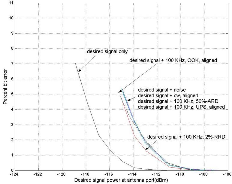
Figure 4.8. Percent bit-error versus variable LMR power for Receiver B in P25 mode – 100-kHz PRF UWB interference.
