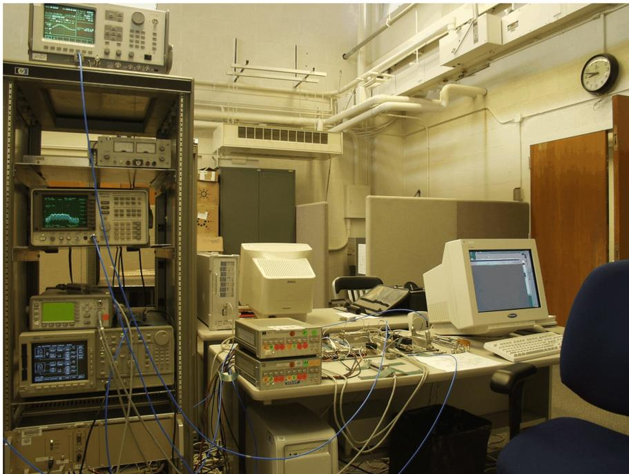
Figure 3.1. Public Safety radio interference test bed.
