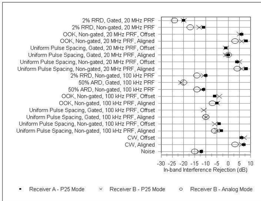
Figure 4.1. In-band interference rejection ( $P_{REF} - P_I$ ).
