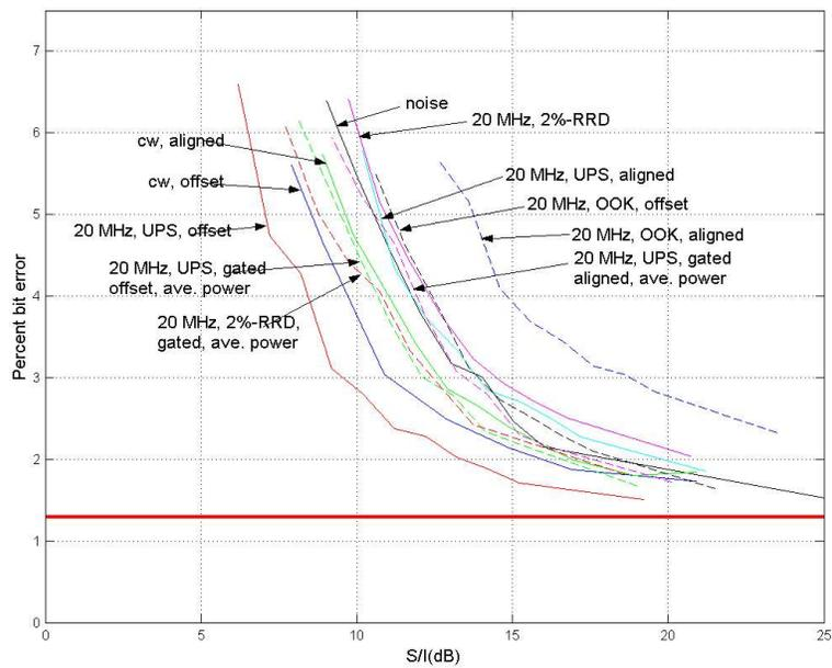
Figure 4.15. Percent bit-error versus S/I for Receiver A in P25 mode – 20-MHz PRF UWB interference.
