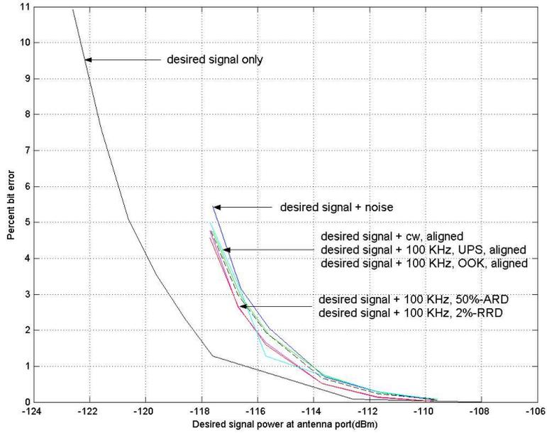
Figure 4.4. Percent bit-error versus variable LMR power for Receiver A in P25 mode – 100-kHz PRF UWB interference.
