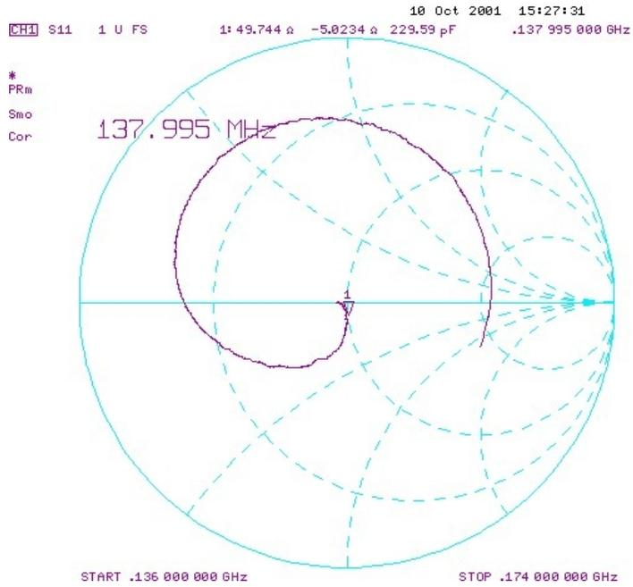
Figure 3.4. Input impedance to receiver A as seen at the input to the matching stub.
