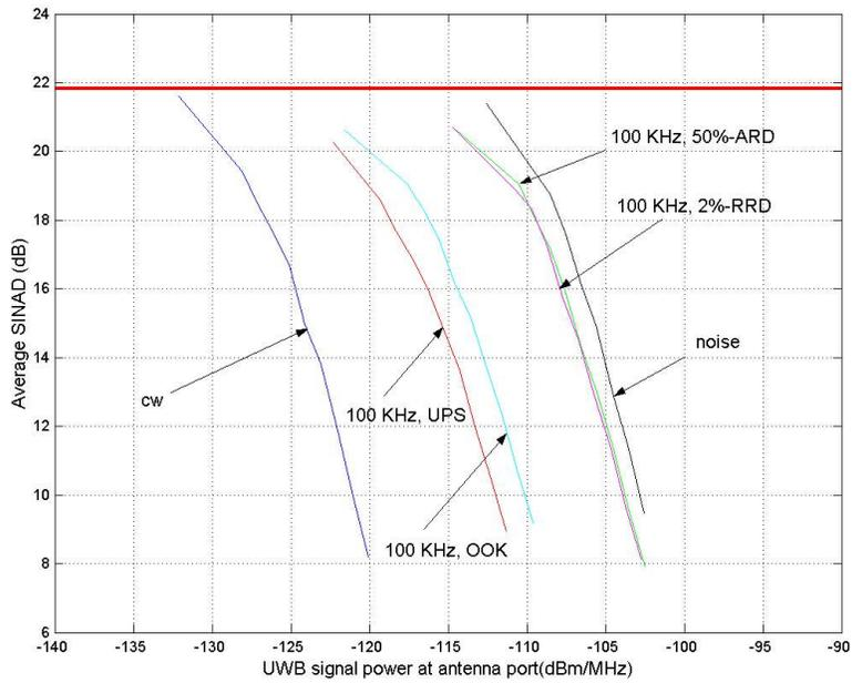
Figure 4.10. Average SINAD versus variable interference power density for Receiver B in analog mode – 100-kHz PRF UWB interference.
