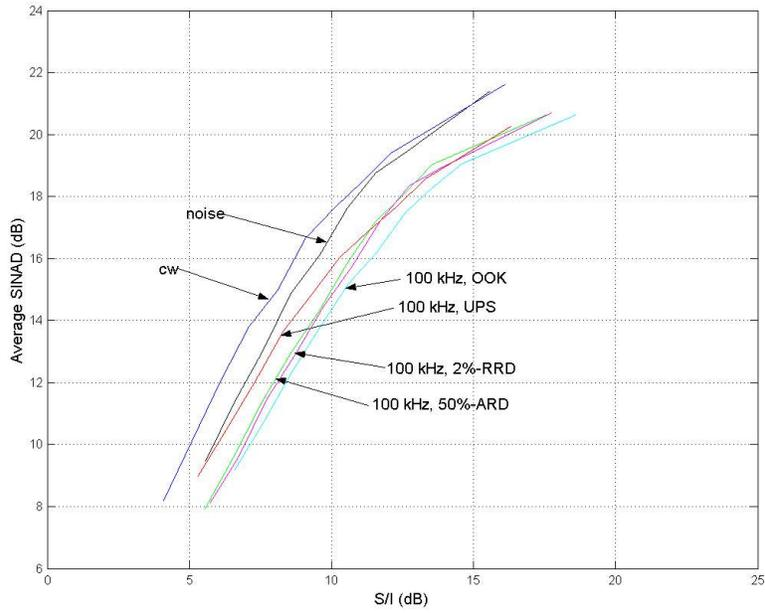
Figure 4.18. Average SINAD versus S/I for Receiver B in analog mode – 100-kHz PRF UWB interference.
