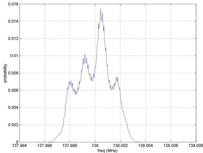
Figure 3.3. Frequency histogram of the C4FM modulated signal.
