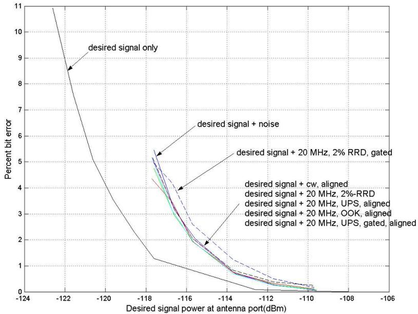
Figure 4.5. Percent bit-error versus variable LMR power for Receiver A in P25 mode – 20-MHz PRF UWB interference.
