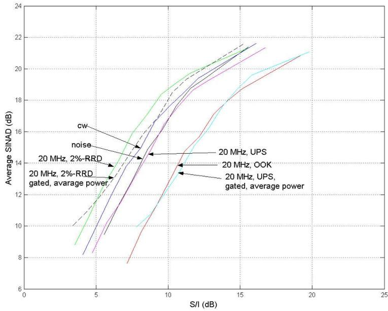
Figure 4.19. Average SINAD versus S/I for Receiver B in analog mode – 20-MHz PRF UWB interference.
