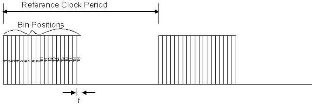
Figure A-1. Discrete binning of pulse position for clock referenced dithering .
