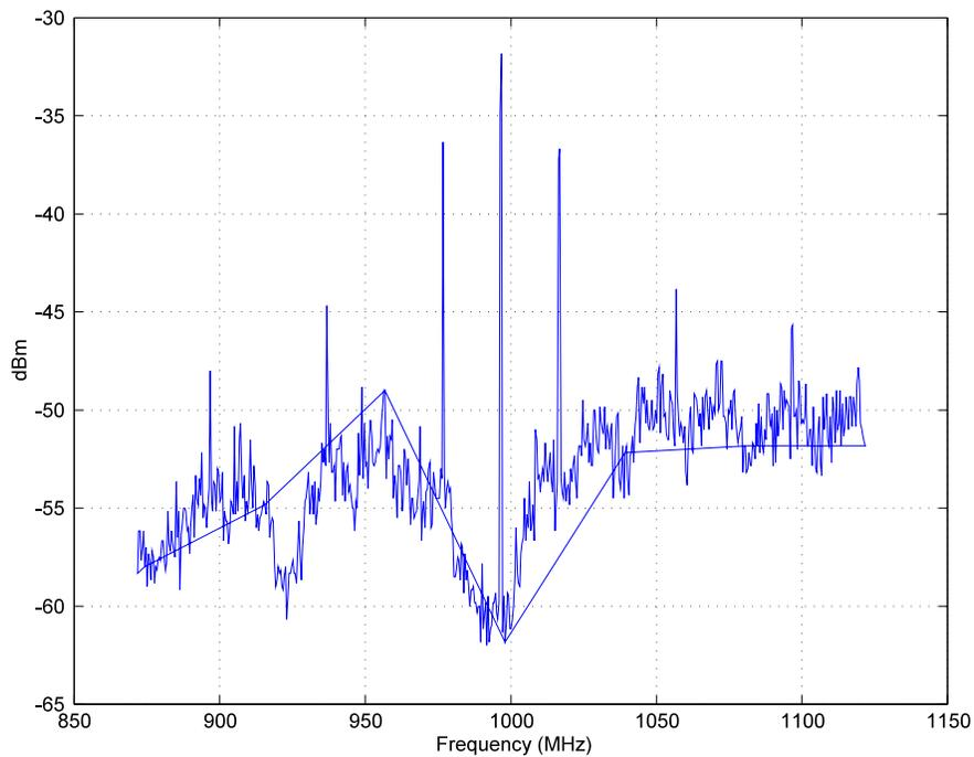
Figure A.3. Spectral lines due to discrete binning of pulse position.
