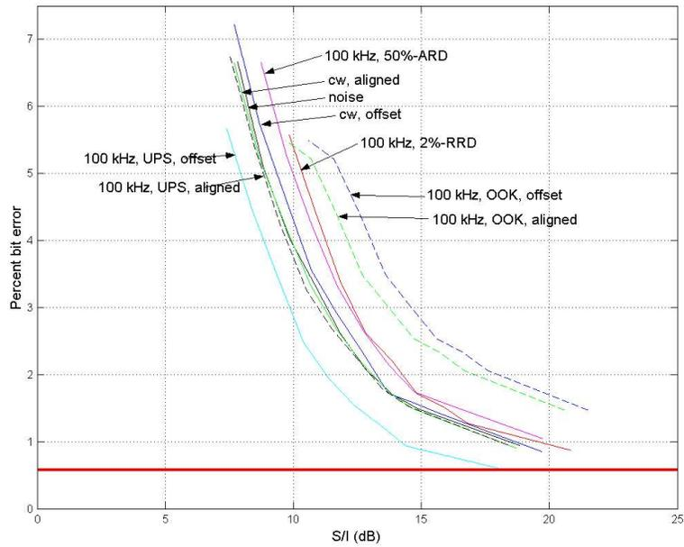
Figure 4.16. Percent bit-error versus S/I for Receiver B in P25 mode – 100-kHz PRF UWB interference.
