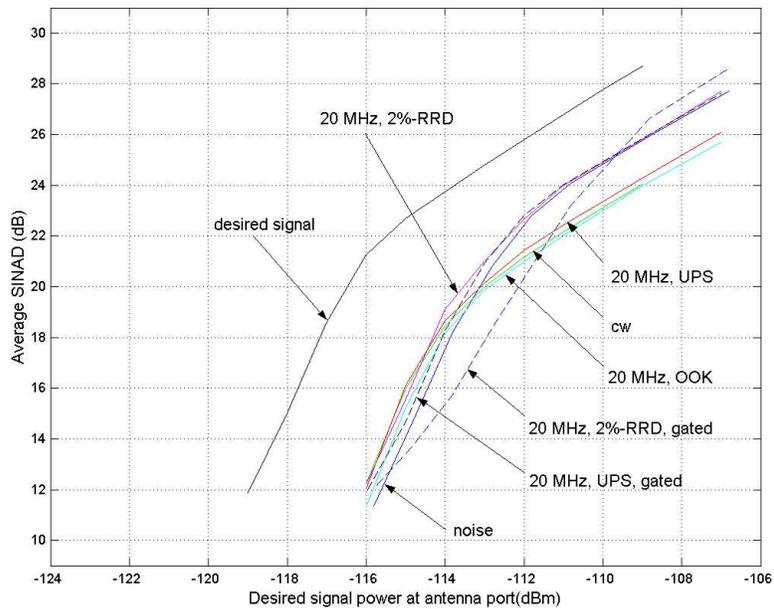
Figure 4.13. Average SINAD versus variable LMR power for Receiver B in analog mode – 20-MHz PRF UWB interference.
