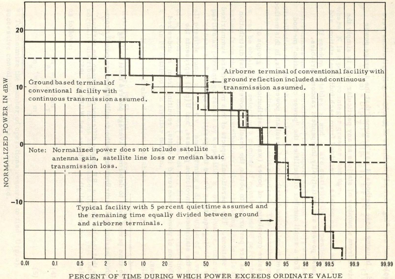
Figure 2. Development of power distribution for typical facility.
