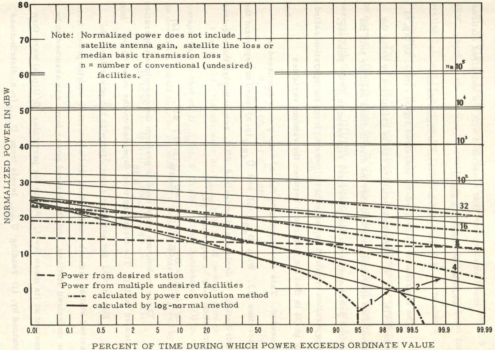
Figure 3.  $U_{dBW}(p, n)$  at satellite terminal.
