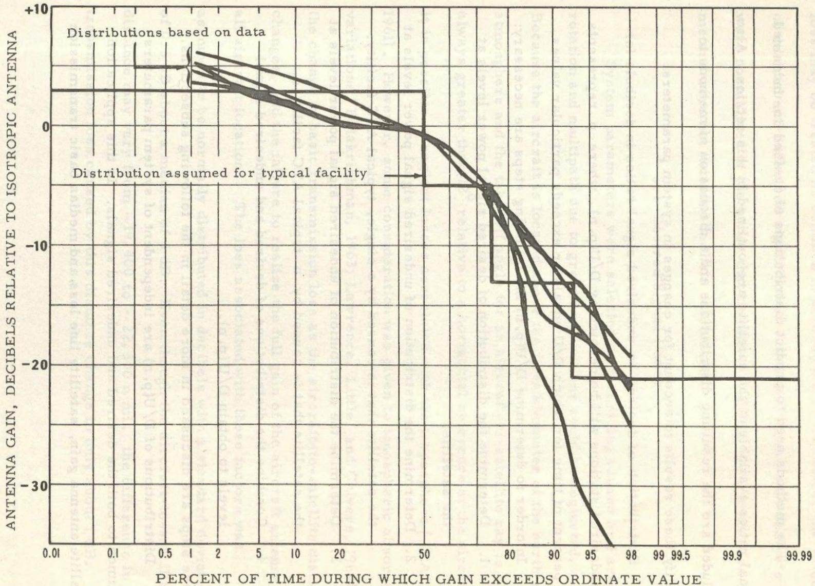
Figure 1. Distribution of aircraft antenna gain for typical facility.
