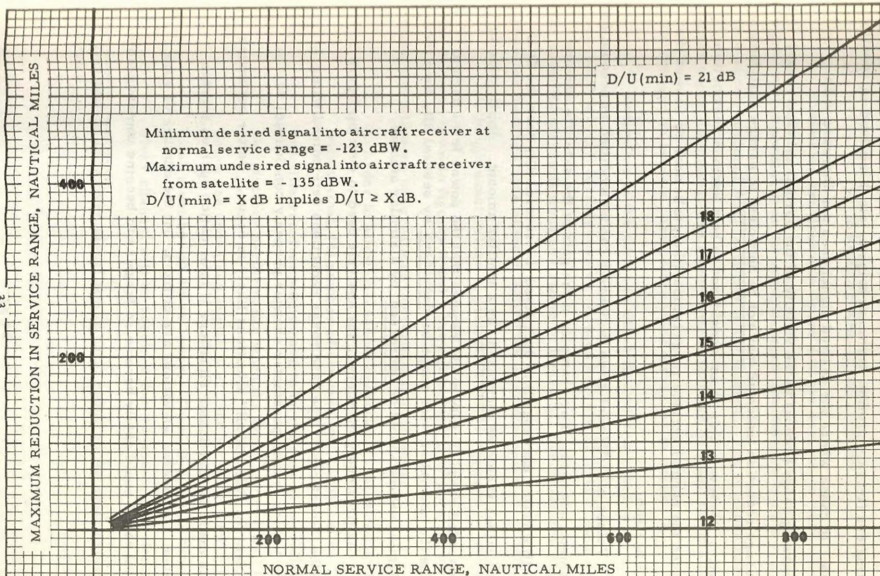
Figure 5. Conventional ATC facility service range reduction due to interference from satellite.
