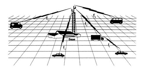
Figure 1. One-frequency non-repeater simplex mobile system.
