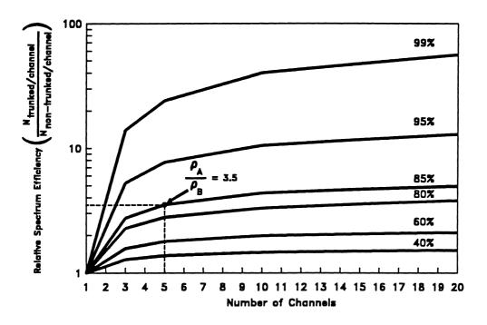
Figure A-2. Comparison of spectral efficiencies of N-channel systems without a control channel with single channel systems.
