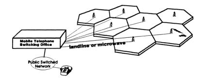
Figure 4. Cellular telephone system.
