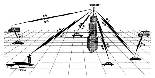
Figure 2. Repeater system with mobile-to-mobile capability.
