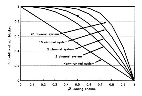
Figure A-1. Probability of access not being blocked for various systems with equal perchannel loading. The trunking characteristics assume a M/M/m queuing process without a control channel.<sup>52</sup>
