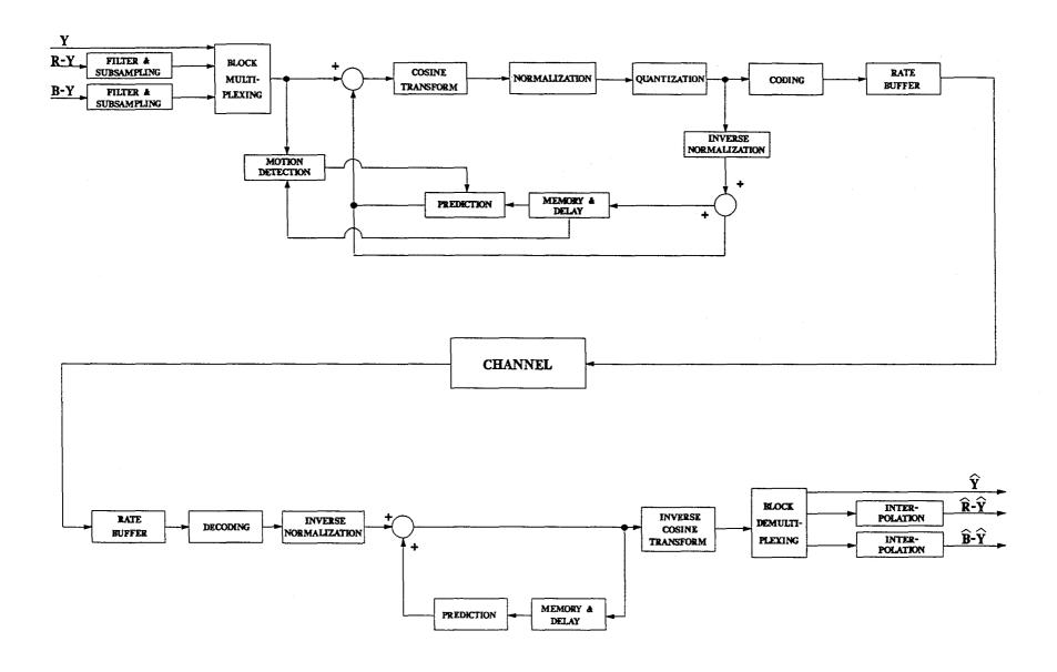
Figure 6. Combined interframe and intraframe scene adaptive coding system (as in Chen and Hein, 1987).
