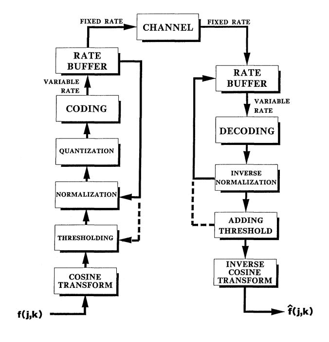
Figure 5. Basic diagram of the scene adaptive coder (from Chen, 1981).
