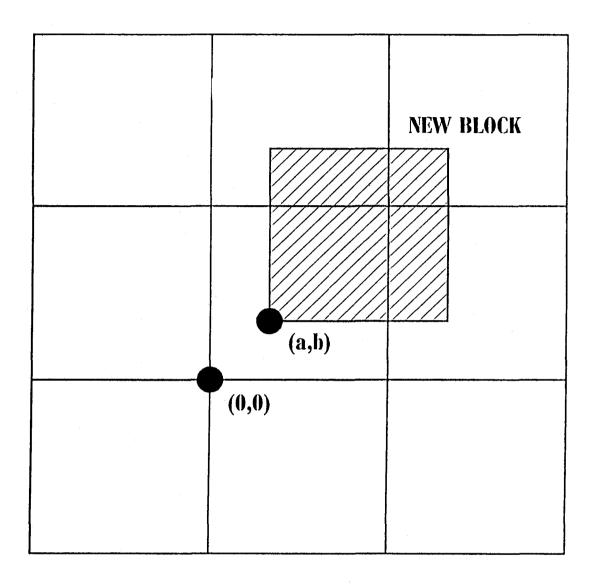
Figure 4. The role of displacement vector (a,b) in block matching.
