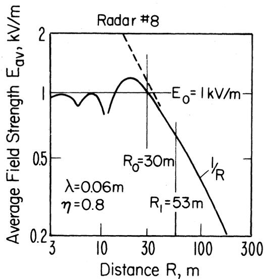
Figure 8. Measured on-axis electric near field strength from 300 to 3 m approaching radar #8 (Table 2) (Glaser and Heimer, 1971).
