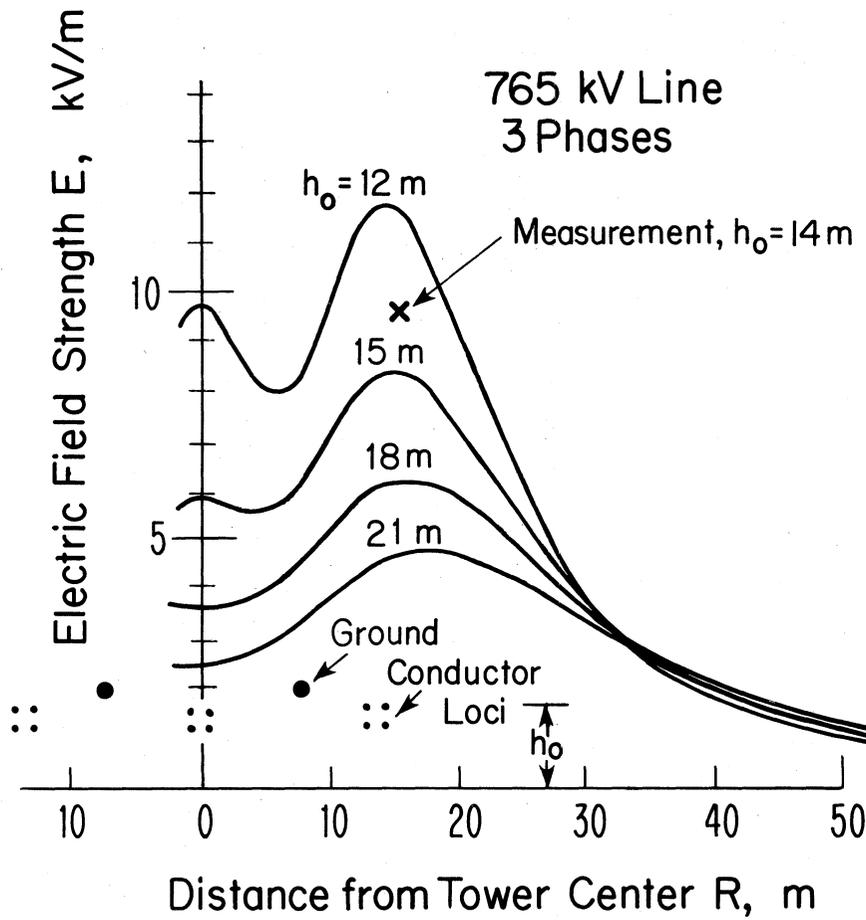
Figure 9. Calculated electric field strength profile at ground level (1 m) for 765 kV line (Tell et al., 1977).
