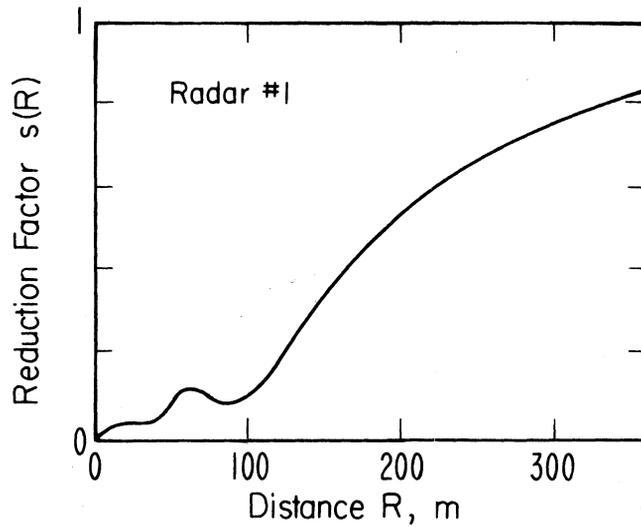
Figure 7. Computer near-field gain reduction factor for uniform aperture illumination from 300 to 1 m approaching radar #1 (Table 2) (Larsen and Shafer, 1977)
