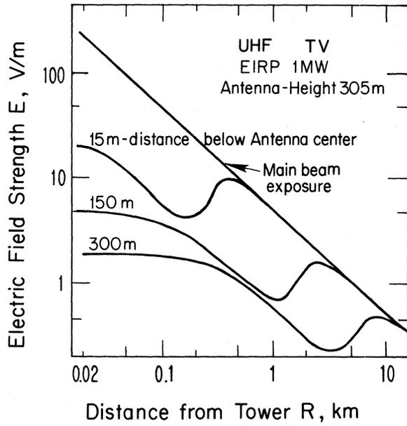
Figure 3. Electric field strength of UHF TV station (Tell and Janes, 1976).
