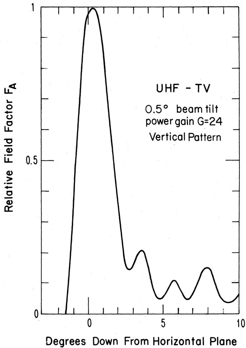
Figure 2. Vertical radiation pattern of typical UHF TV antenna (Tell and Janes, 1976).
