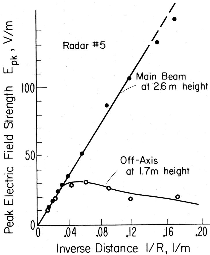
Figure 6. Measured on-axis and off-axis electric field strength from 100 to 5 m approaching radar #5 (Table 2) (Larsen and Shafer, 1977).
