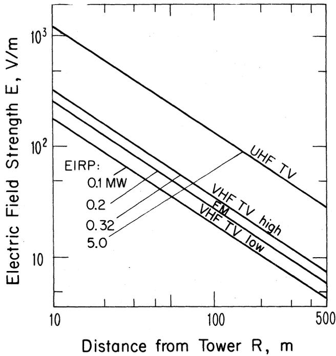
Figure 4. Maximum free-space electric field strength from FM and TV broadcasting (equations 1, 6) for main beam exposure.
