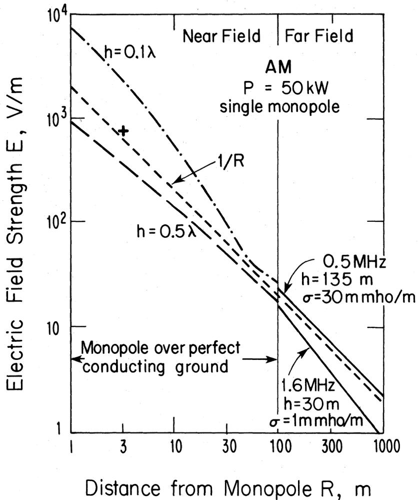
Figure 1. Ground-level electric field strength estimates for a 50 kW AM broadcast station employing a single monopole antenna. + Measured (Adams et al., 1977); near field calculations (Tell and Janes, 1976); far field (Berry, 1978).
