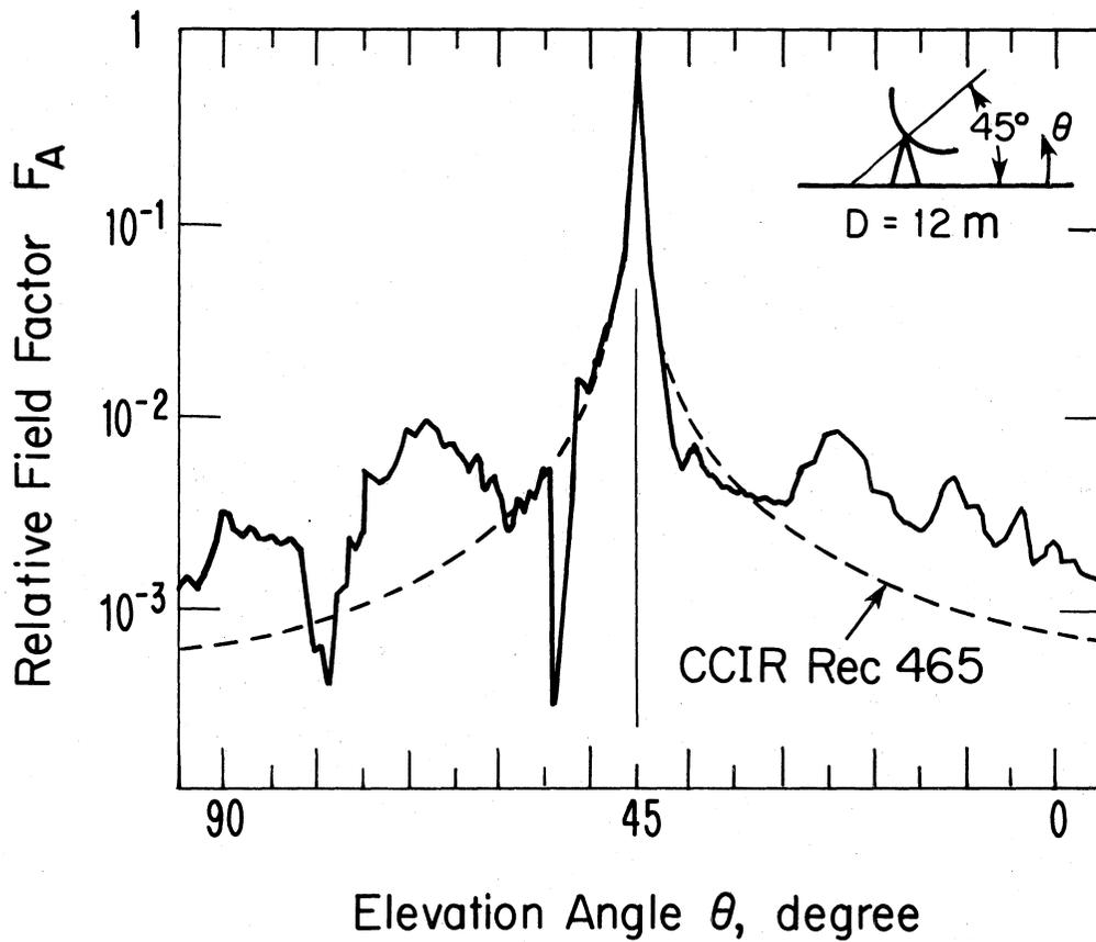
Figure 5. Measured sidelobe structure of a  $D = 12\text{ m}$  reflector antenna operating around 4 GHz.
