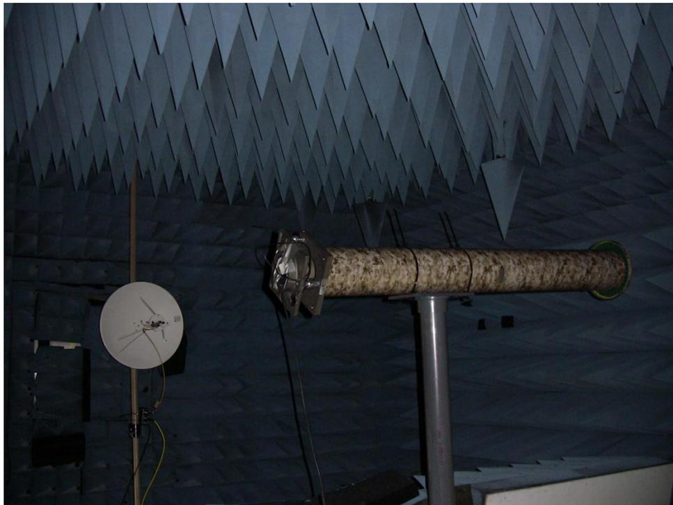
Figure 40. Elevation pattern measurement setup in the anechoic chamber.
