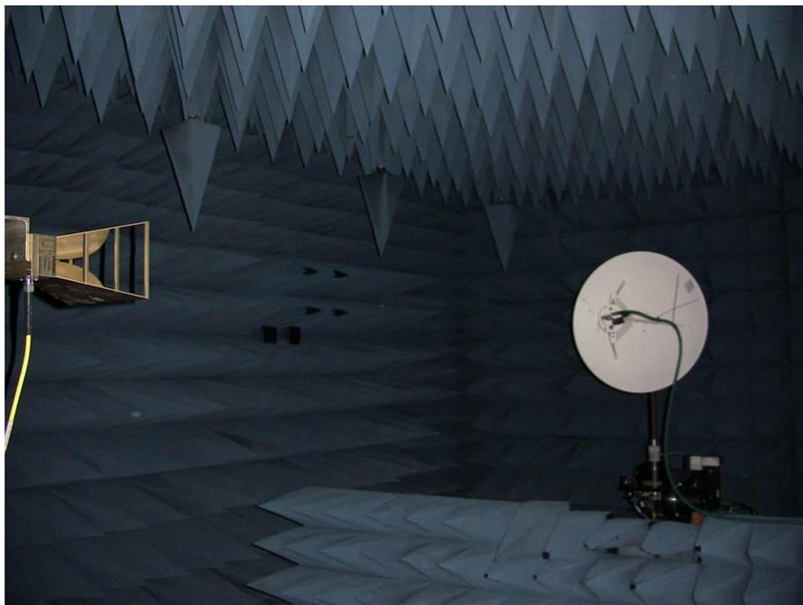
Figure A-6. Insertion measurement between a DRH and parabolic dish antenna.
